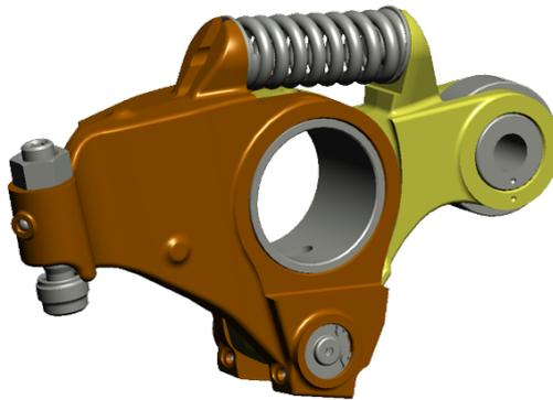
Figura 8.6. Exhaust rocker arm
