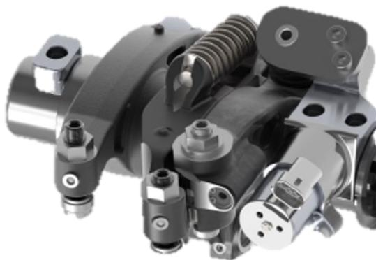
Figura 8.11. HP engine brake
