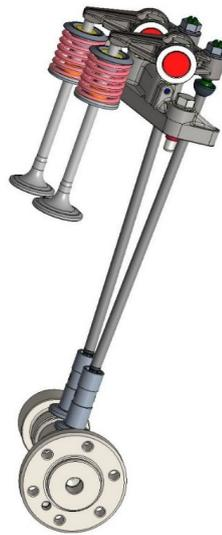
Figura 6.3. Center pivot rocker arm with pushrod - traditional version
