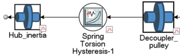
Figure 7.6: Decoupler model in GT-Ise
