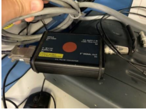
Figure 8.5: Signal multiplier used for bench testing
