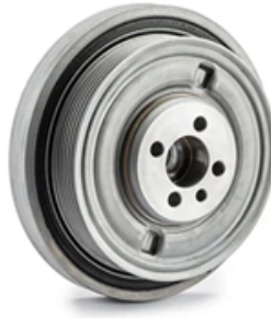
Figure 2.25: Example of decoupler from DAYCO [14]
