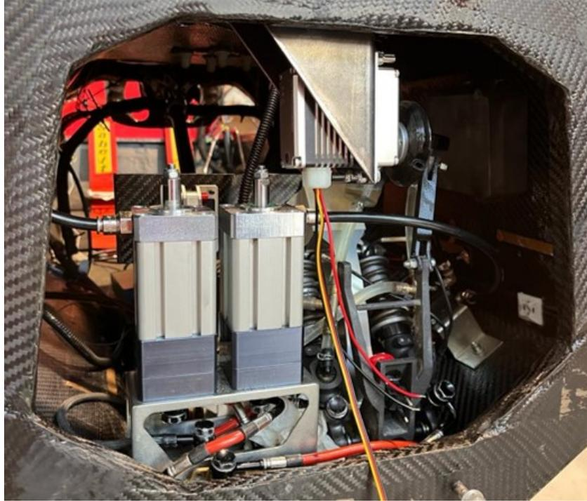
**Figure 2.5:** EBS (left) and ASB (top right) mounted on the vehicle
