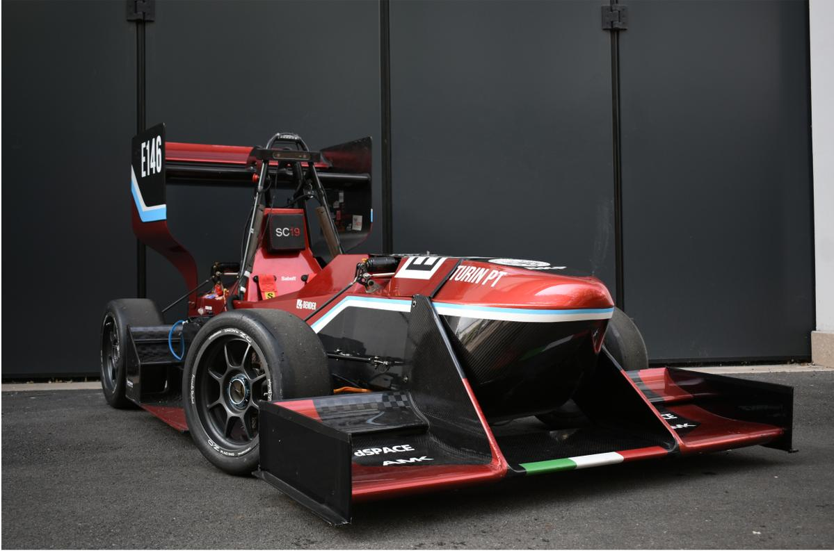
**Figure 1.3:** SC19 Formula Student Electric prototype
