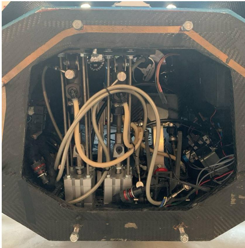
**Figure 5.1:** SCD23 EBS mounted on the vehicle
