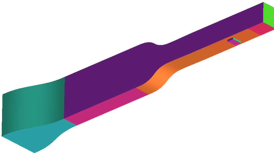
Figure 4.1: Wind tunnel with cavity section.
