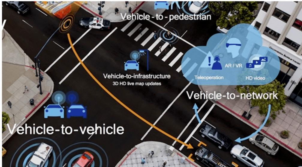
**Figure 2.3:** Different communication of vehicle
