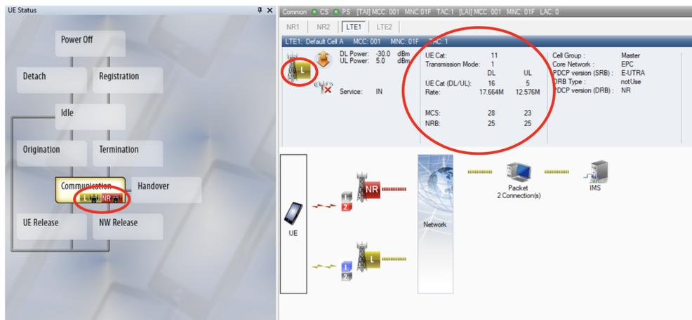
Figure 4.12: Multi-cell network connection after handover in EN-DC mode
