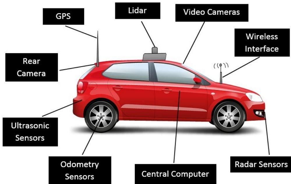
**Figure 2.2:** Autonomous vehicle components
