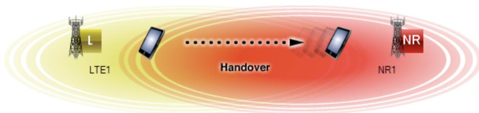
Figure 4.9: Handover and connection with the NR cell
