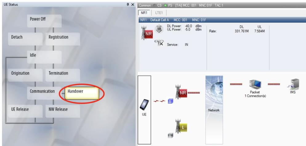
Figure 4.8: Handover and connection with the NR cell
