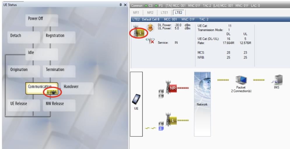
**Figure 4.10:** Multi-cell network connection before enabling EN-DC mode
