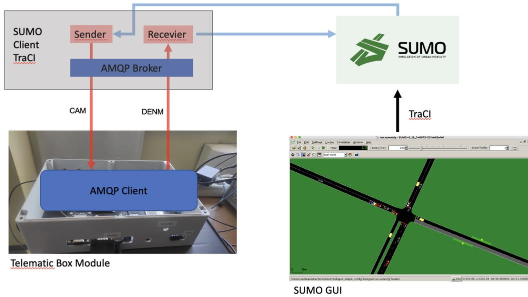
Figure 5.2: High level SUMO Client architecture
