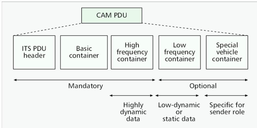
**Figure 2.4:** Structure of a CAM message
