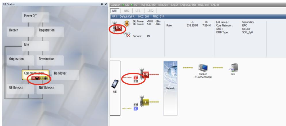
**Figure 4.11:** Multi-cell network connection after enabling EN-DC mode
