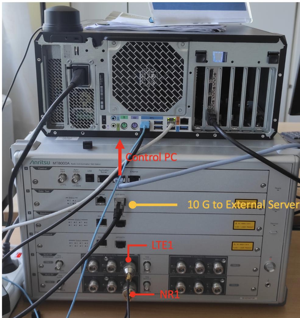
**Figure 4.5:** MT8000A connection for LTE and NR
