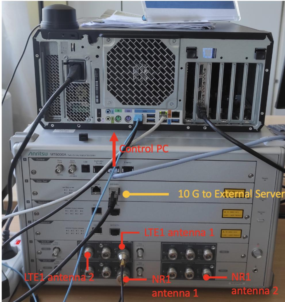
Figure 4.18: MT8000A connection for MIMO 2x2
