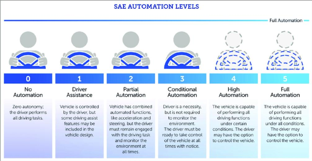
Figure 2.1: SAE Automation levels
