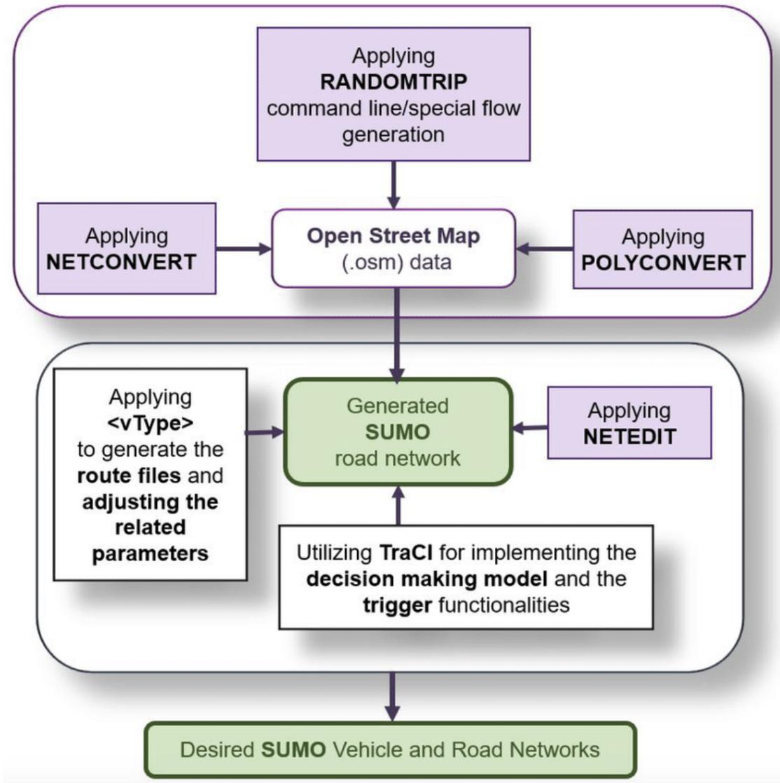
Figure 6.2: SUMO network building procedure
