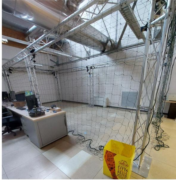
Figure 3.5: *The used safety cage for drone flight*
