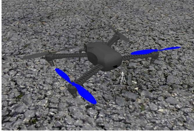
Figure 5.4: *Model of the Iris drone used in the Gazebo simulation. The white lines in the front represent the field of view of the camera.*
