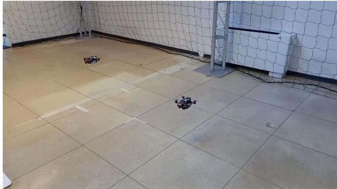
Figure 5.6: *Drones in flight during the test of the flocking algorithm.*
