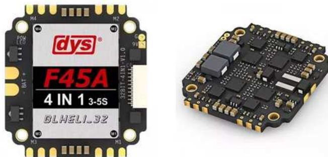
Figure 2.6. Electronic Speed Controller model showing the back (right side) and the front (left side).
