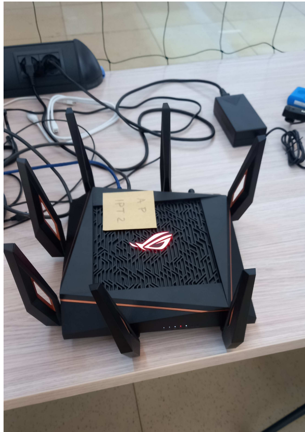
Figure 2.18. Model of the WiFi router used to connect the CGS via the VICON system and with the drones
