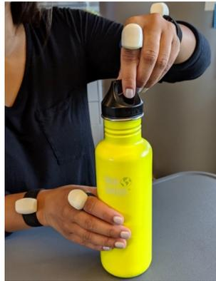
**Figure 1.1:** Displays the proposed finger-worn sensor and ring-sensor.
