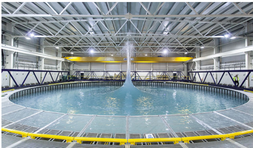
Figure 1.3: Example of a mid size paddle activated wave tank. The wave shape can be precisely tuned by controlling the paddles array [3]
