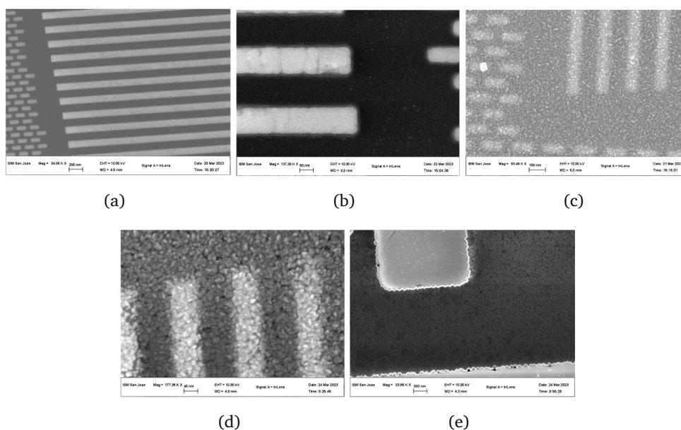
**Fig. 5.2:** (a) 50 ZnO ALD cycles, (b) 114 ZnO ALD cycles, (c) 200 ZnO ALD cycles, (d) 150 ZnO ALD cycles on P, (e) 150 ZnO ALD cycles on K
