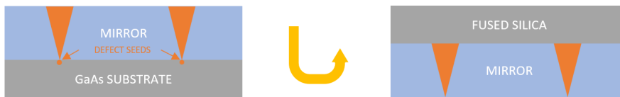
Figure 18: The layered mirror structure is initially grown on a GaAs substrate. Following this, the mirror coating is separated, inverted, and positioned on an optically fused silica substrate. This process is informed by the fact that optical absorption primarily occurs in the initial few layers exposed to the laser, and the top layers grown are anticipated to be of lower quality. An instance justifying this assumption involves the potential growth of a pyramidal-shaped crystalline defect through the layers, which could initiate in the first layer and expand significantly towards the end of the deposition process. Particularly in the case of AlGaAs, the formation of a crystalline Aluminum cluster could serve as a point absorber for the mirror.
