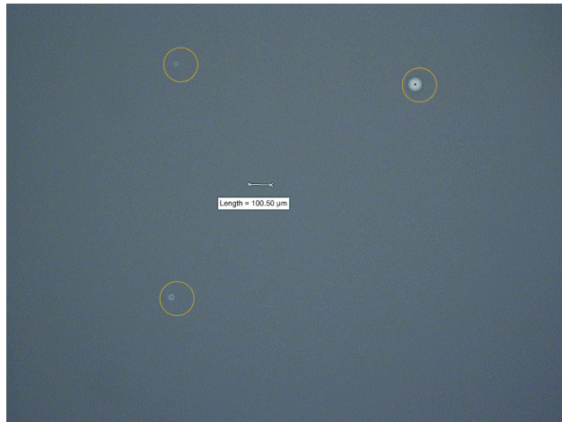
Figure 26: This photograph, captured from the rear side of the sample, reveals multiple impacted points. The same conical shape discussed in Figure 25b is apparent, supporting the direct correlation between the damage to the mirror layers and the power-dependent measurements conducted on the sample.
