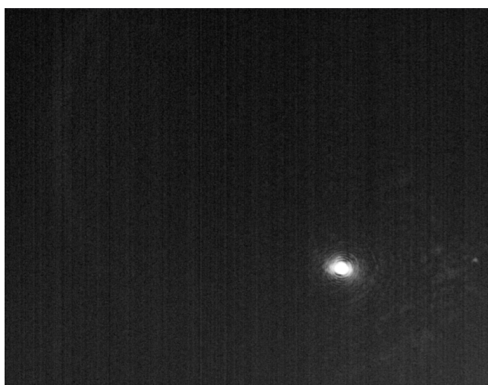
Figure 3.29: This IR camera acquisition shows a round laser spot with circular lobes of the \text{PSF}^2 .
