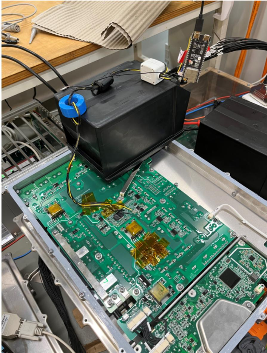
**Figure 5.10:** Test setup with on-board charger and ferrite beads
