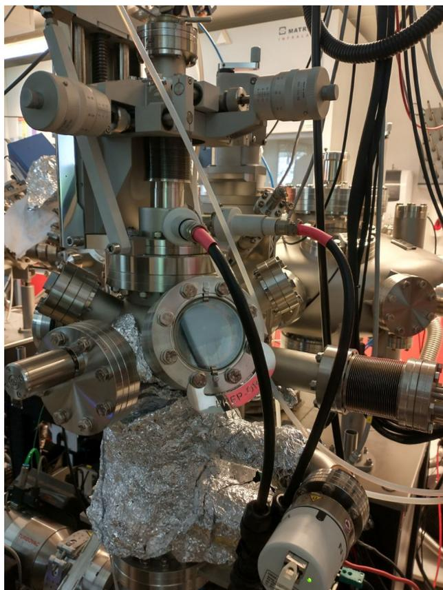
Figure 7.1. Picture of the organic deposition chamber.
