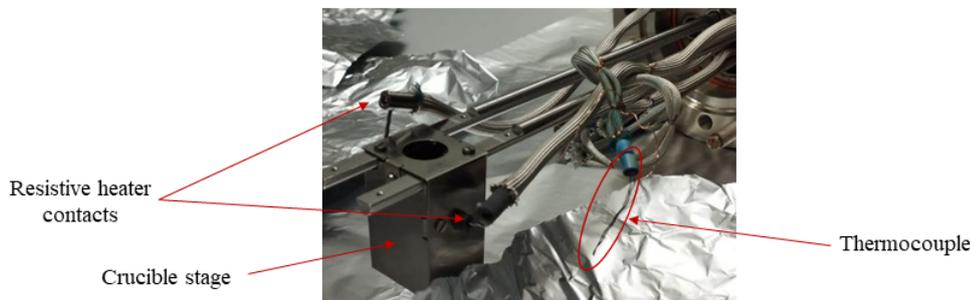
Figure 6.6. Picture of the crucible stage and the thermocouple filament.
