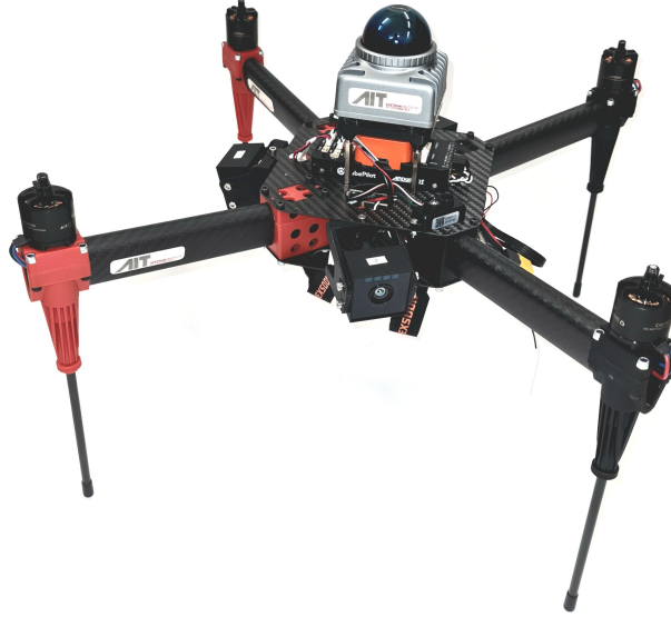
Figure 4.8: UAV mounting the Livox Mid360
