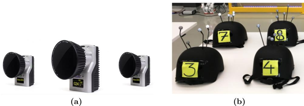
**Figure 4.5:** (a) Qualisys Oqus 7+ infrared cameras; (b) helmets with reflective markers, used to track pedestrians.
