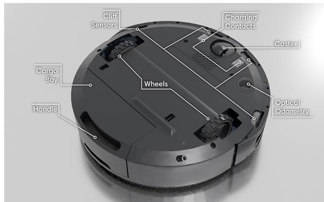
**Figure 5.3:** Bottom view of the Create3 mobile base.
