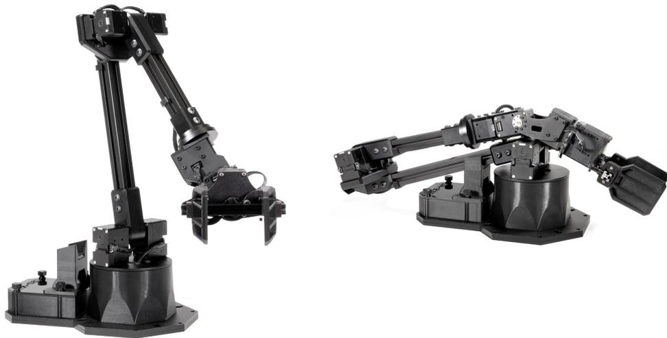
**Figure 5.5:** WidowX-250 6DOF Robot arm.
