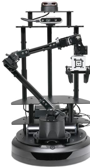
**Figure 5.1:** Mobile robot Locobot WX250s-6DOF used in the simulation campaign
