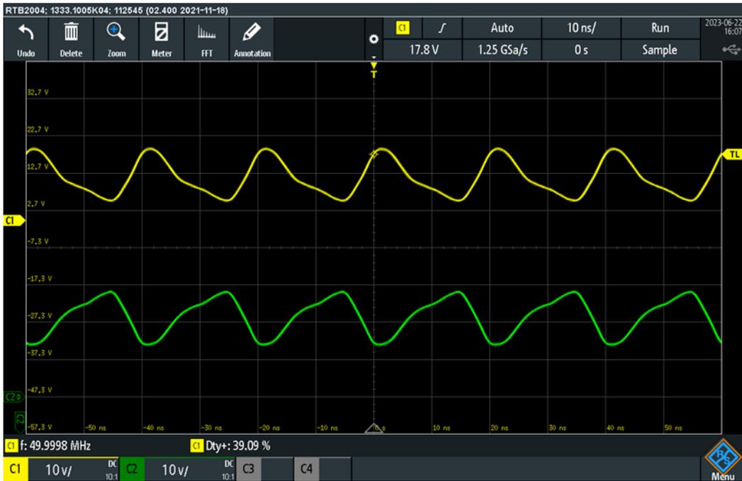
Figure 5.19: 50 MHz signal and 50% duty cycle
