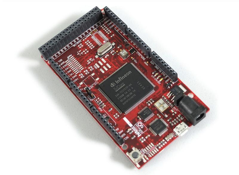
**Figure 2.1:** 32 bit AURIX Tricore Microcontroller [4]
