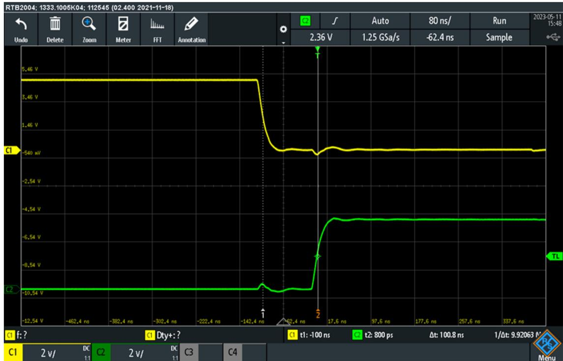
Figure 5.5: Oscilloscope view of dead time insertion detail
