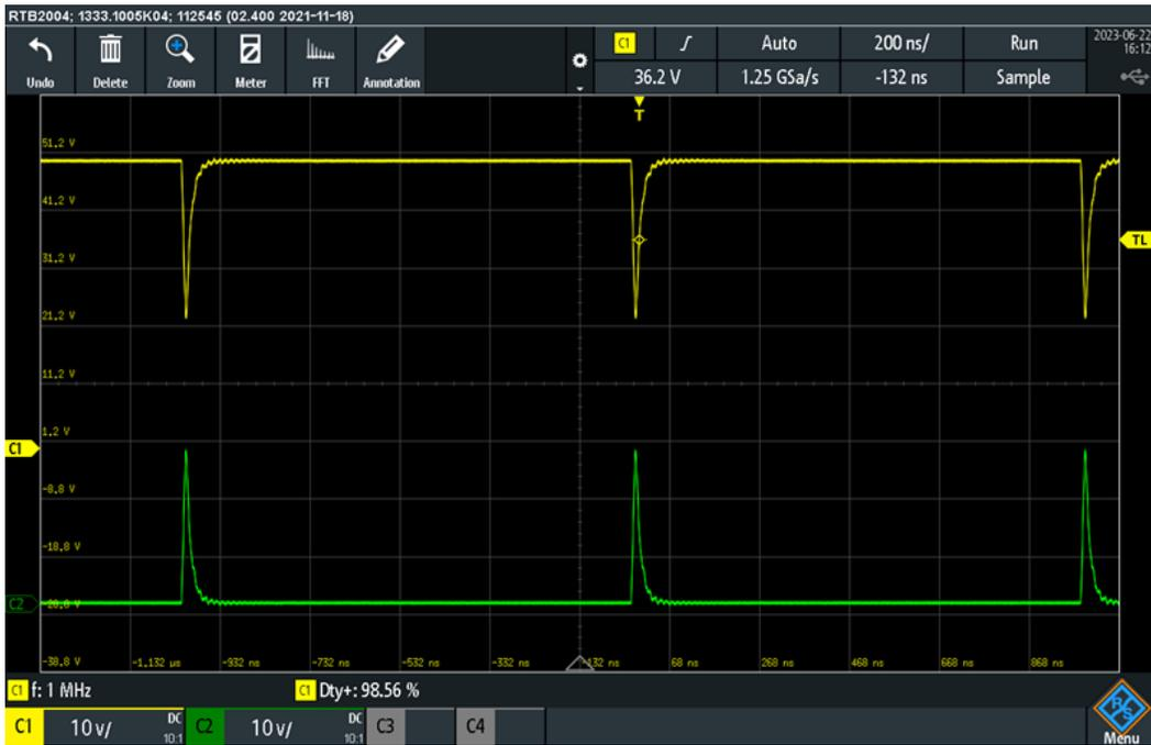
Figure 5.11: 1 MHz signal and 99% duty cycle
