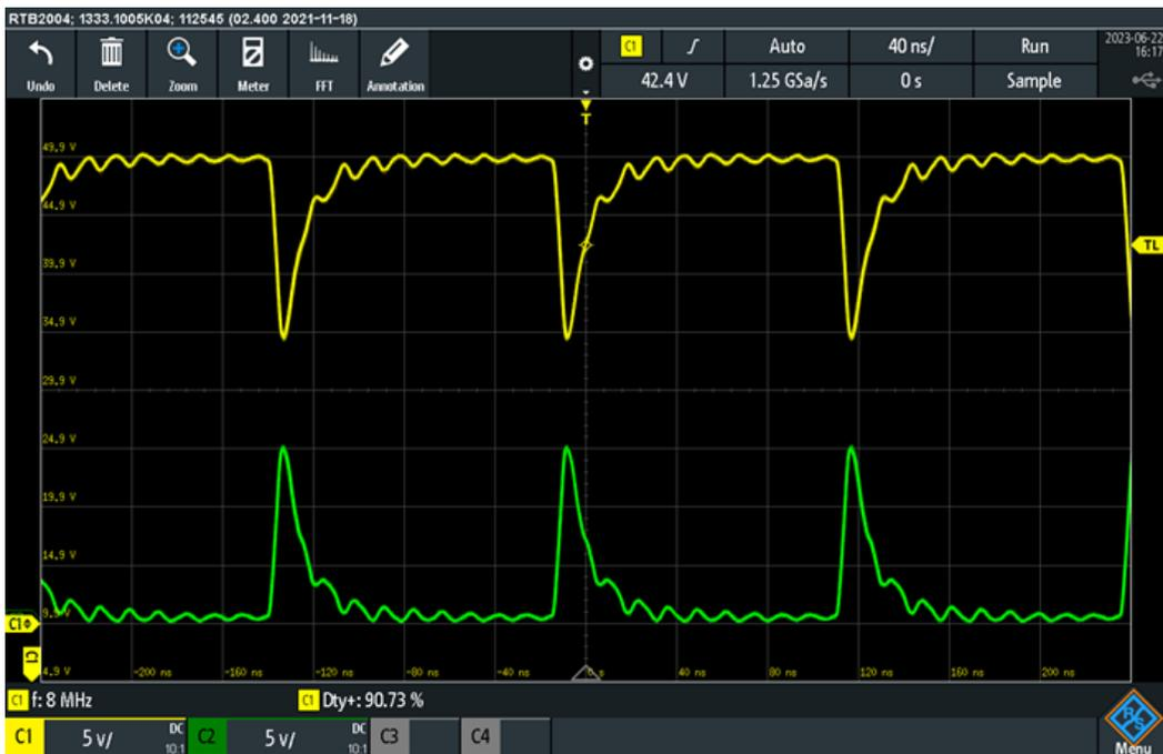
Figure 5.17: 8 MHz signal and 90% duty cycle
