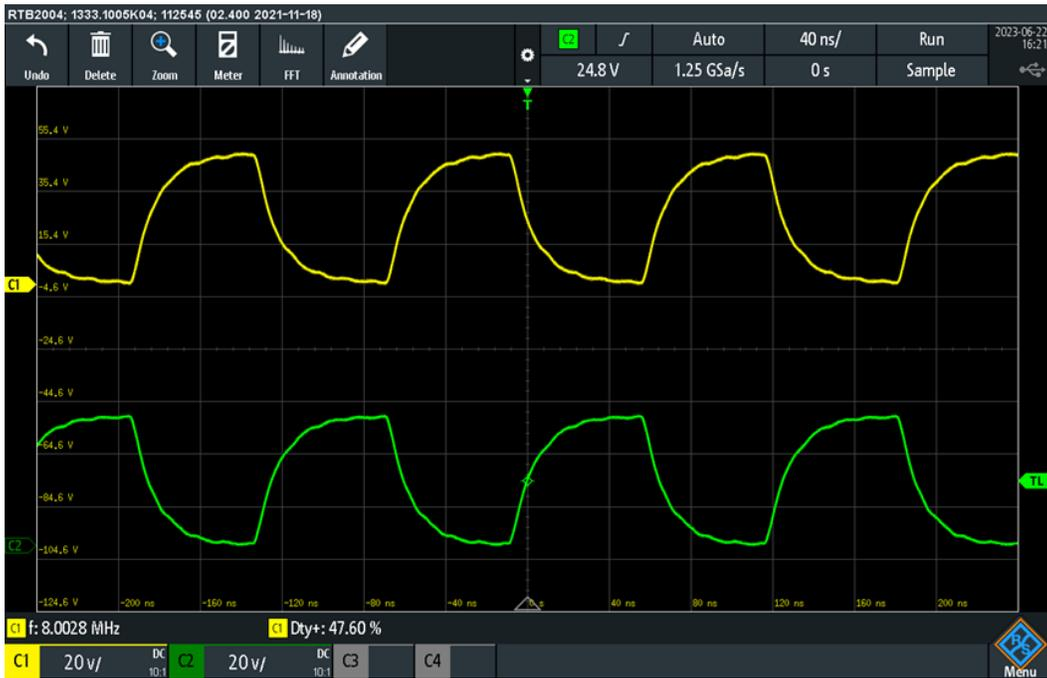
Figure 5.16: 8 MHz signal and 50% duty cycle
