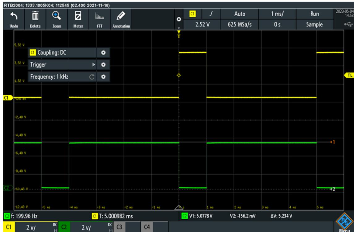
**Figure 5.2:** Oscilloscope view of signals for standard PWM generation
