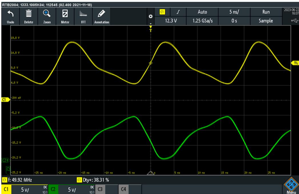
Figure 5.20: Detail of 50 MHz signal and 50% duty cycle
