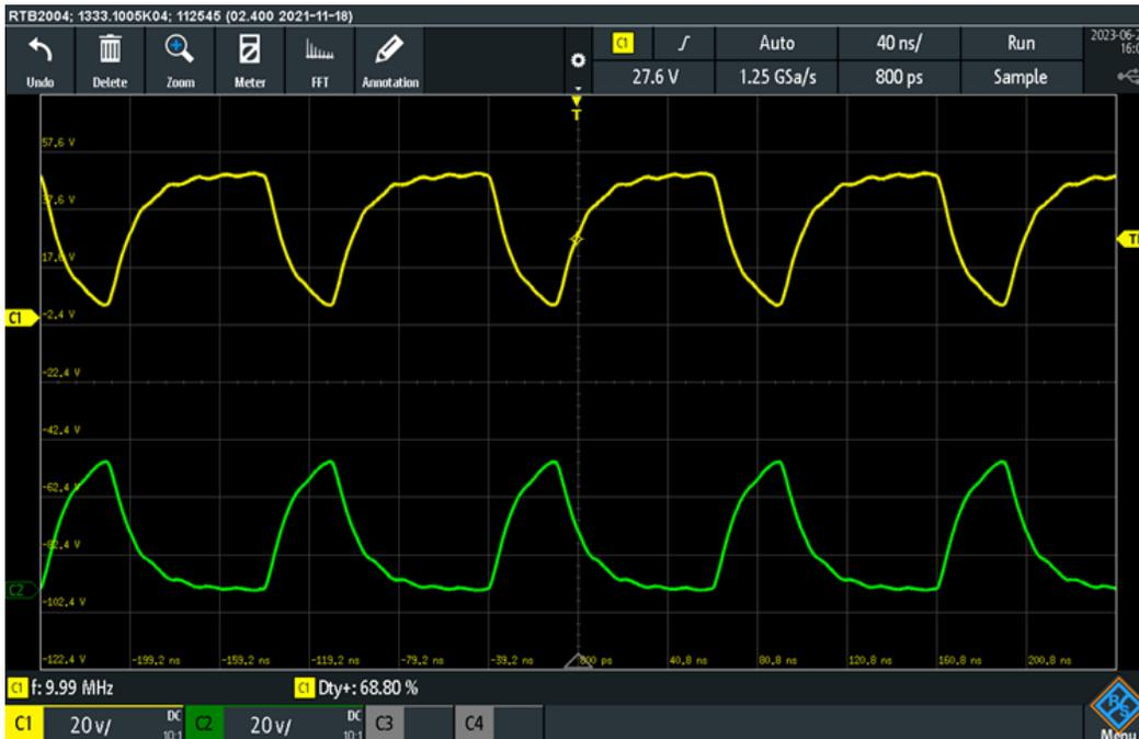
**Figure 5.18:** 10 MHz signal and 80% duty cycle
