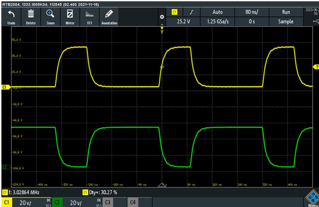
Figure 5.13: 3 MHz signal and 30% duty cycle
