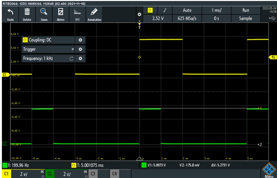
**Figure 5.3:** Oscilloscope view of edge aligned signals
