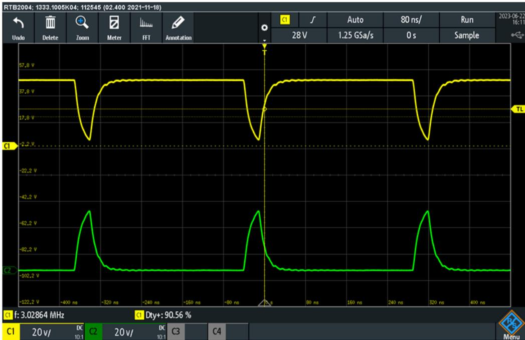
**Figure 5.14:** 3 MHz signal and 90% duty cycle
