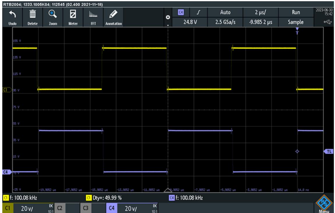
**Figure 5.7:** Shift of  $1/2$  between signals
