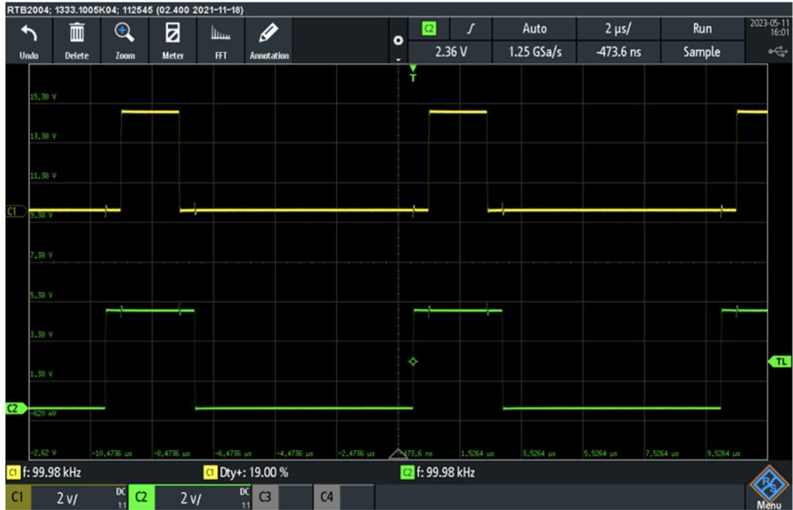
Figure 5.9: Center alignment example with up counter
