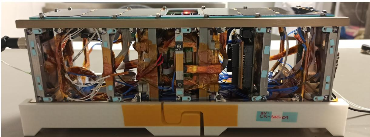
**Figure 7.19:** The integrated flight model without the last two solar panels.
