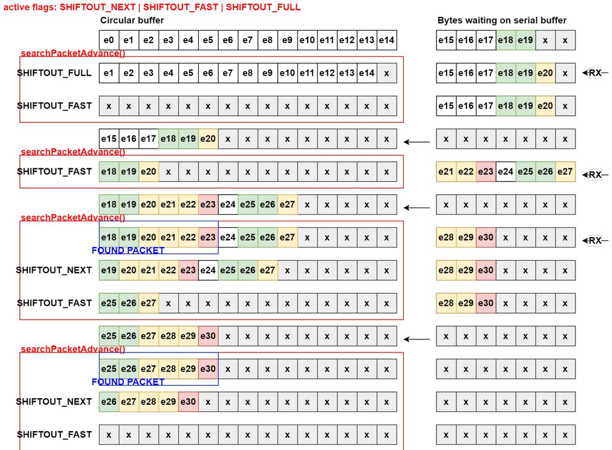
**Figure 6.21:** Real-case example of searchPacketAdvance() applied to an incoming stream of data. Head bytes are in green, tail bytes are in red. Function calls are represented as red squares around the circular buffer, function flags that cause the buffer to advance on each step are shown on the left.
