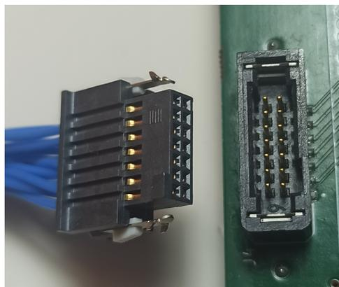
Figure 5.32: Samtec ISDF-07-D-M cable housing (left) and TFM-107-02-S-D-WT-P connector (right).
