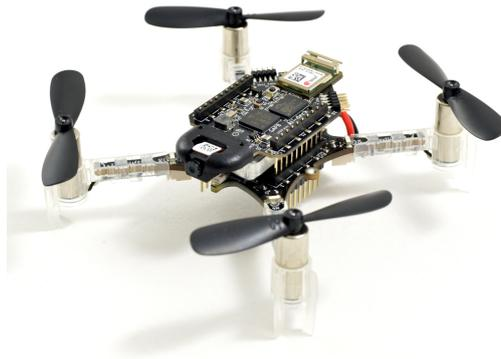
Figure 2.2: The Crazyflie 2.1 with the AI-deck on top. Image from Bitcraze AB [35].
