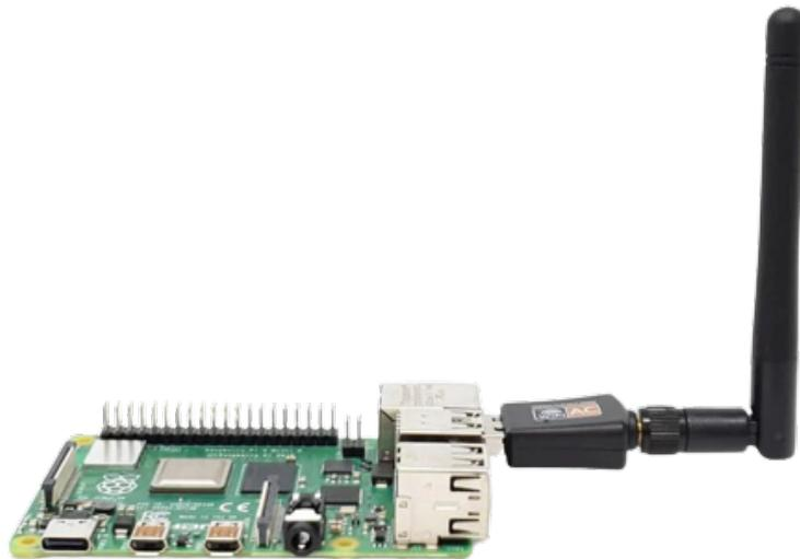
Figure 2.7. A Raspberry Pi board with a WiFi dongle.
