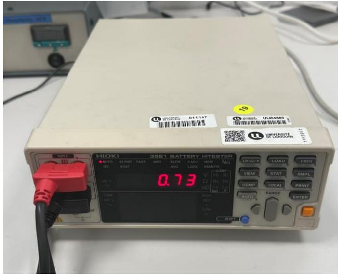
Figure 25 Milliohm meter used in ICR measurements
