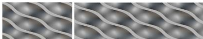
Figure 10: Frontal and lateral view of the Diamond in a 10 mm x 20 mm x 5 mm domain
