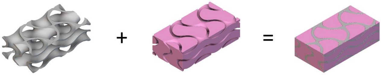
Figure 19: Regions assemblage for the Gyroid in a 10 mm x 20mm x 5mm domain
