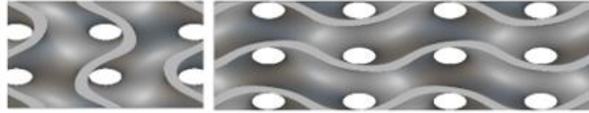
Figure 14: Frontal and lateral view of the Gyroid in a 10 mm x 20mm x 5mm domain
