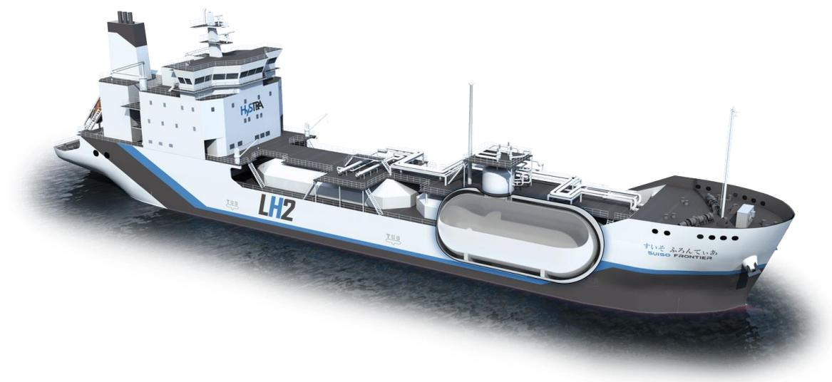
*Figure 3 Suiso Frontier liquid hydrogen tanker [35]*
