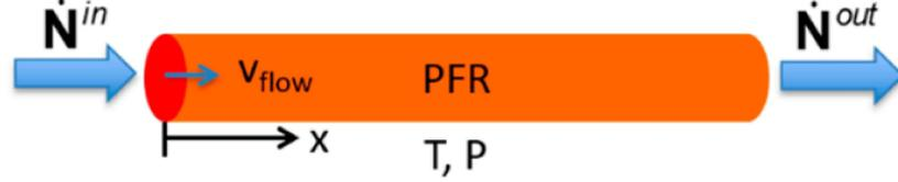
**Figure 2.30:** Scheme of a Plug Flow Reactor, PFR, where reactants flow through a channel, moving at the same velocity and experiencing similar reaction conditions, resulting in efficient and predictable chemical reactions. Image from Terreni et al.(2020).
