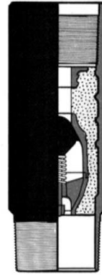
Standard Float Collar with Super Seal Valve. Male and Female Threads Made to Fit Standard API Casing.
