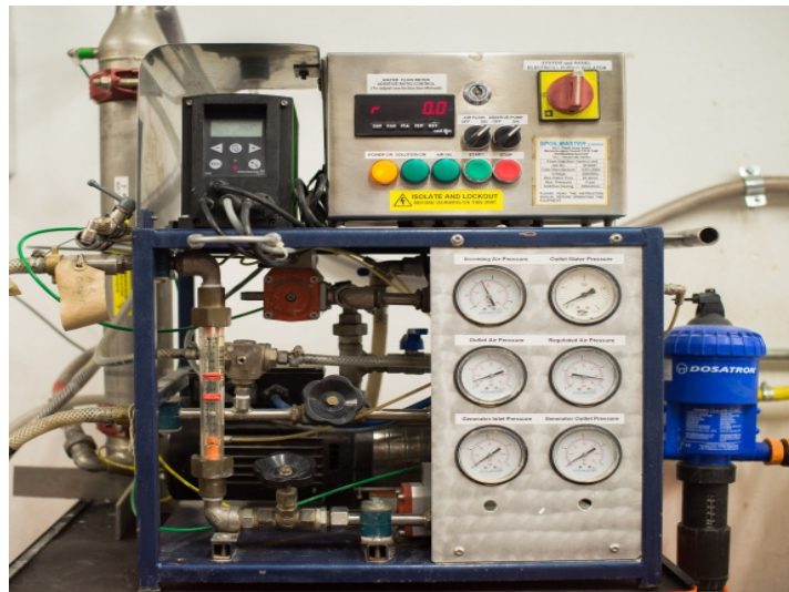
Figure 5_2: Laboratory scale foam generator at TUSC laboratory
