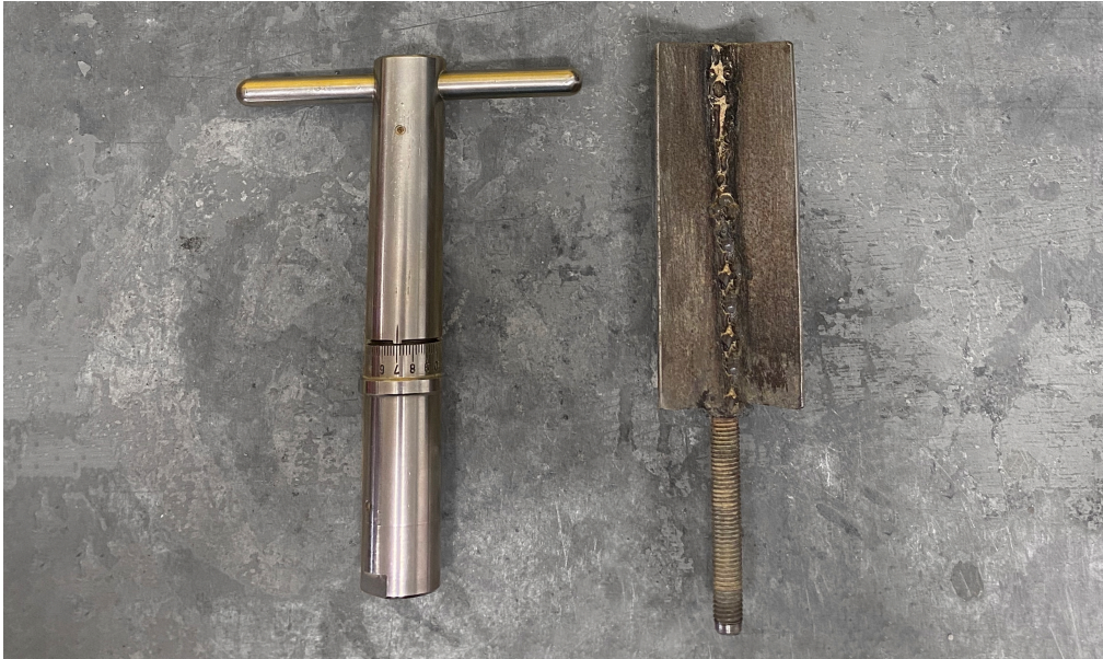
Figure 5_7: Modified vane shear apparatus (Carigi et al., 2020)
