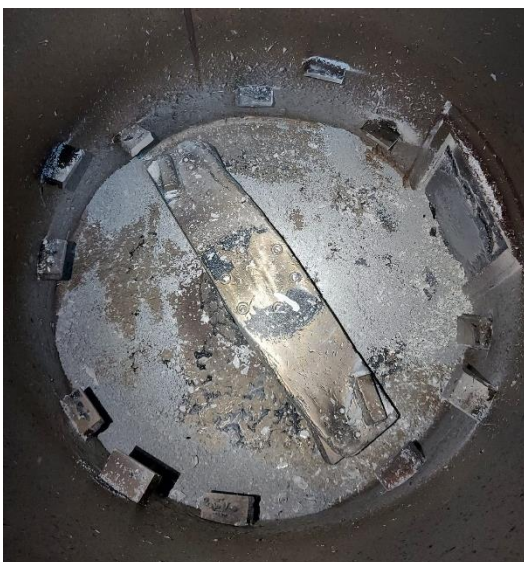
Figure 14 Inside of a densifier
