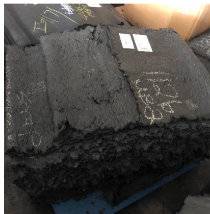
Figure 323 C/D Compound - Masterbatch Source: www.sdpolymers.net
