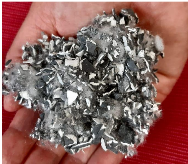
Figure 82 TPO after Grinding Step
