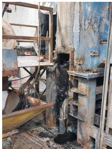
Figure 72 "Melted Pot" during JDR Trial #1
