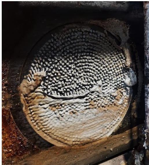
Figure 539 Extruder die after filter blockage during TPO trials.
