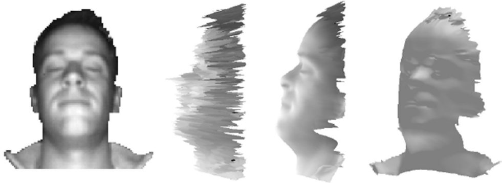
Figure 23 - From left: Intensity image; lateral view of raw measured surface; and surface reconstructed using the shading constraint in lateral and frontal views
