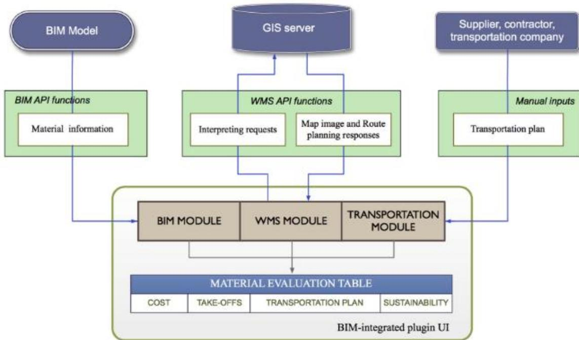
**Figure 3.2.3.2 “Actors connected with BIM integratio”**
