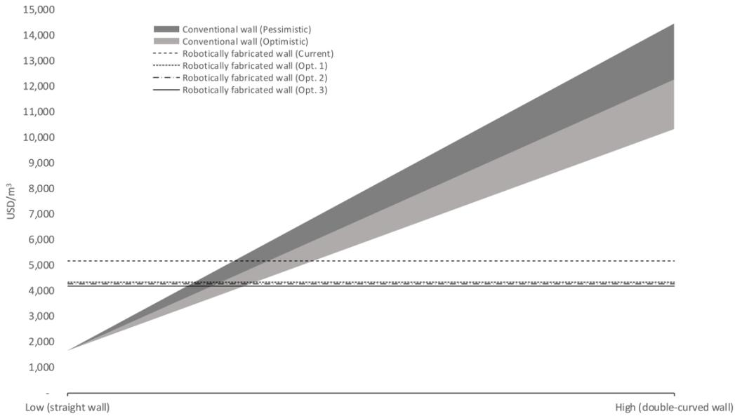
**Figure 3.4.1 “Cost per installed quantity (USD/m3)”**
