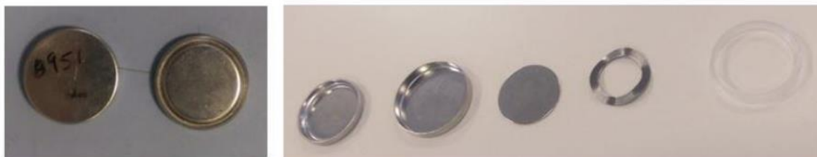
Figure 1.5: Li-S coin-shaped cell structure by IREC
