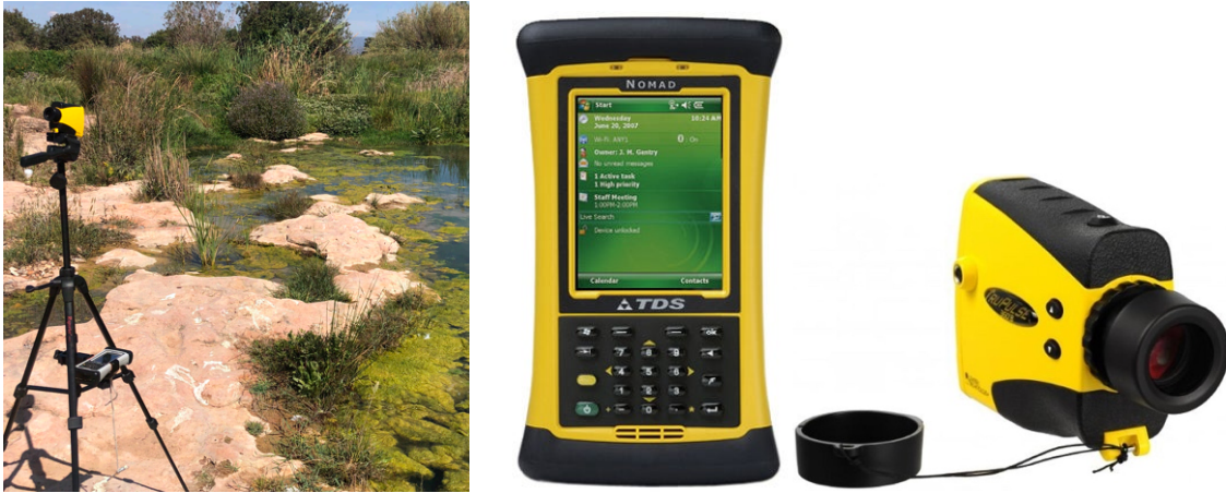
Figure 12: Field survey instrumentations (left) and example of rugged computer (Nomad, center) and laser rangefinder (Lasetech, right)
