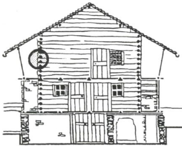
Blockbau structure in house in Alagna; made of larch and fir wood (Mirici Cappa, 1997)
