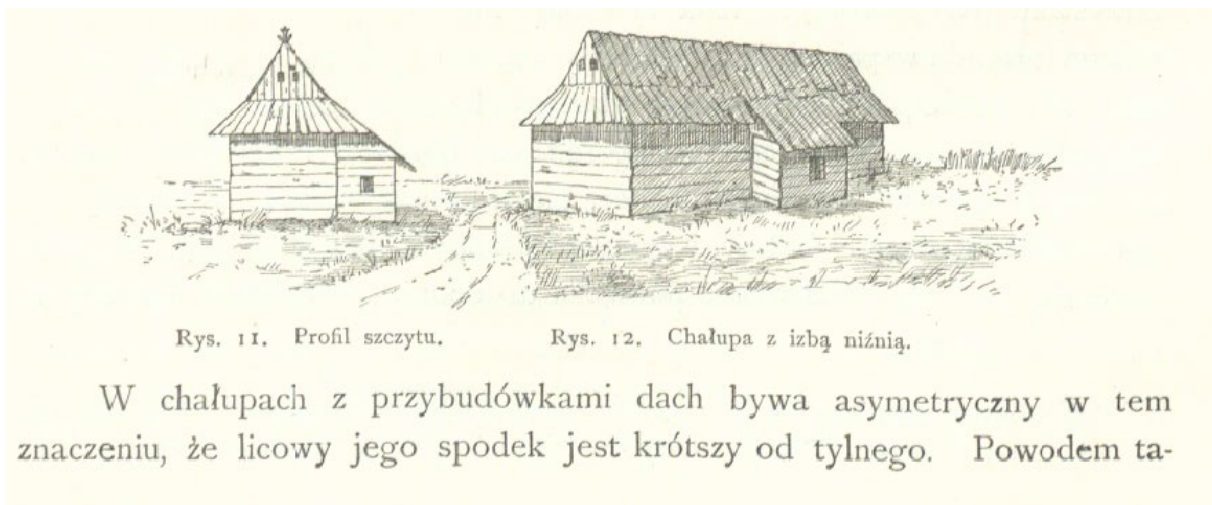
Figure 19 Asymmetric roof in houses with sheds and additional volumes
