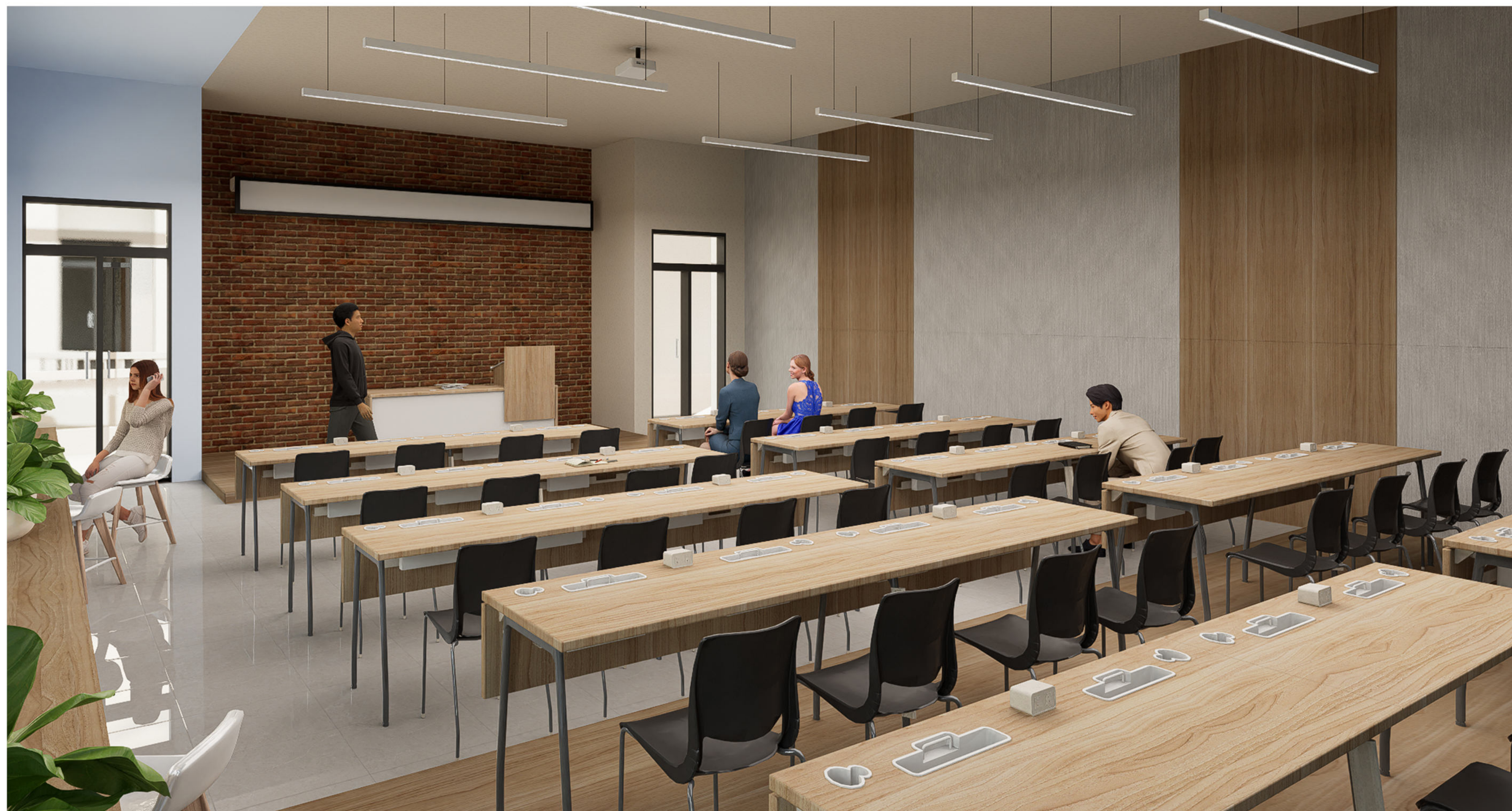
Acoustic panels are placed on 2 walls to minimise external noise which helps with students' focus.
