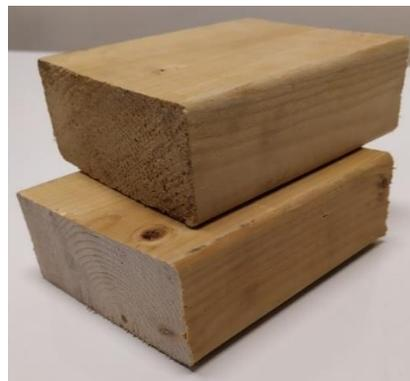
**Figure 3.30** Wooden spacers used in the tests. Approximate dimensions 100x60x35 mm.
