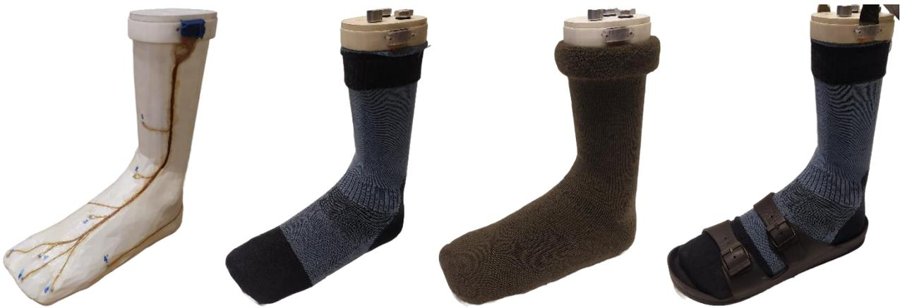
**Figure 3.29** The foot manikin in four different configurations. From left to right: barefoot, wearing a liner, wearing a sock on top of a liner, wearing a liner and a slipper.
