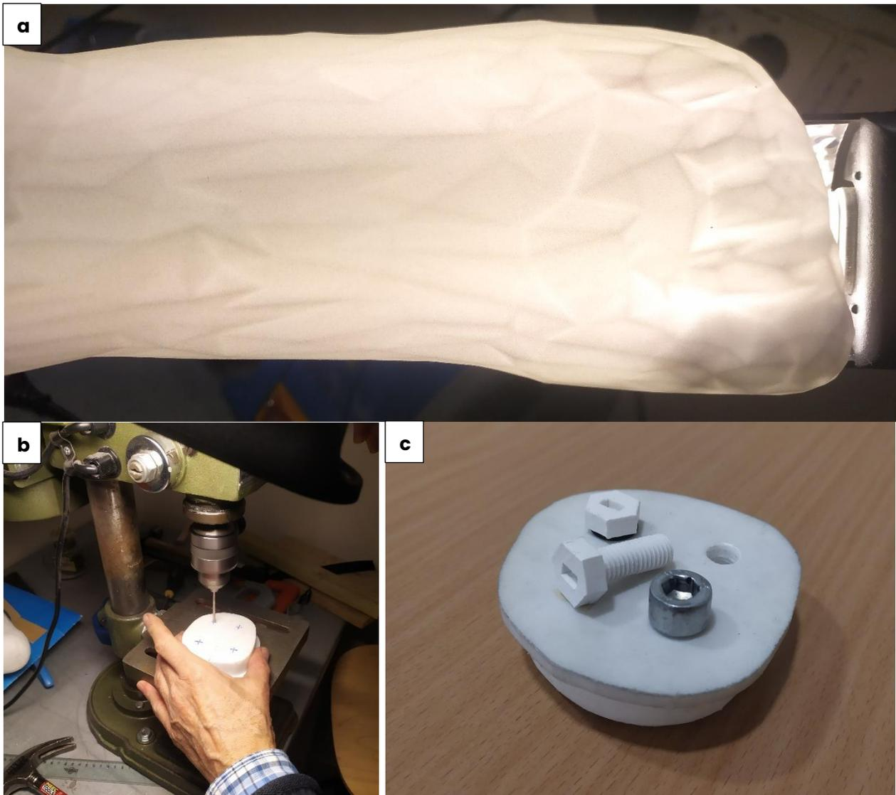
**Figure 3.6** Details of the manikin cleaning and drilling. (a) Dust particles inside the toes, (b) Drilling the plug, (c) The plug with holes and 3D-printed bolts.
