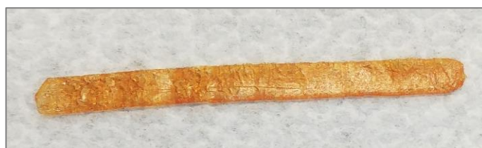
Figure 12: Photo of a BACBDA sample for tensile tests.
