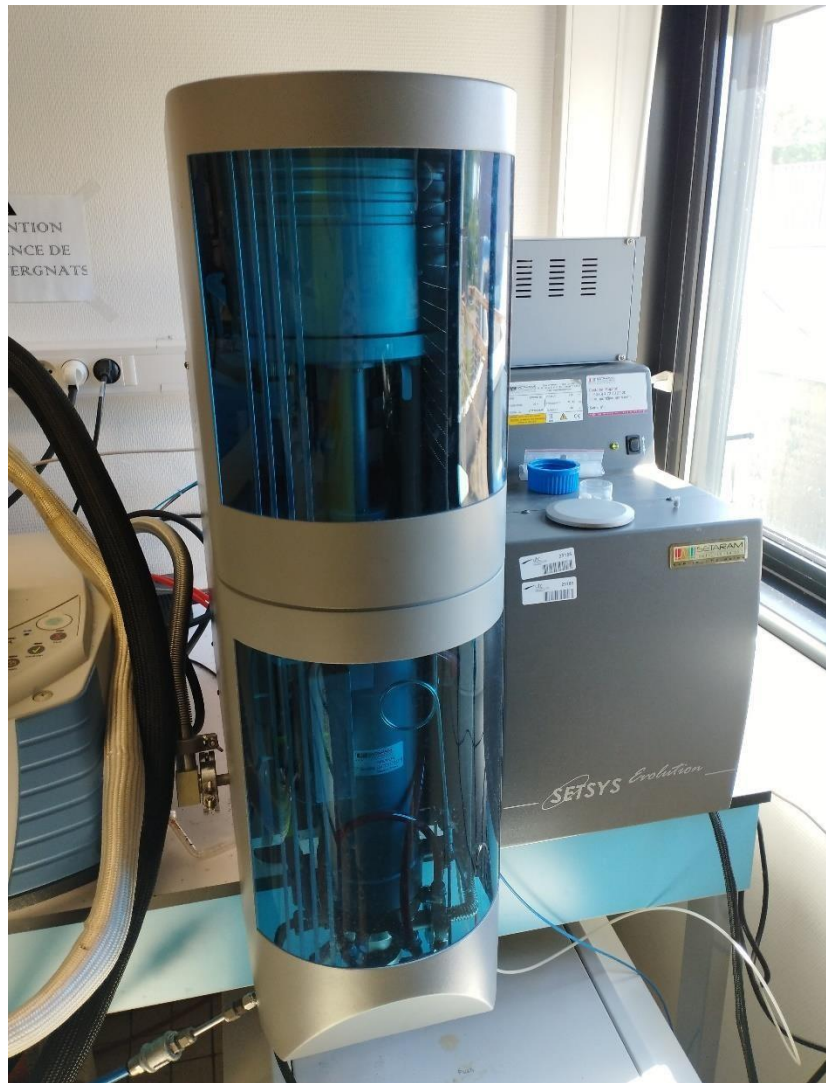
Figure 36: TGA machine in the University of Compiegne, author's elaboration.
