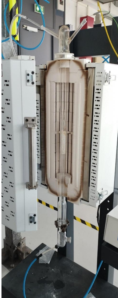
Figure 17: Fixed bed reactor author's elaboration
