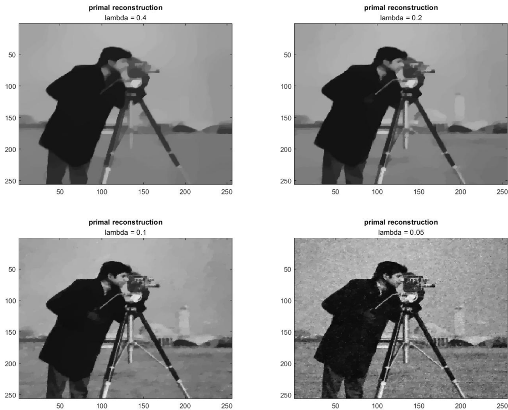
Figure 3.2: Resulting images after applying the ROF minimization with different \lambda/255 : 0.4 (up left), 0.2 (up right), 0.1 (down left), 0.05 (down right).
