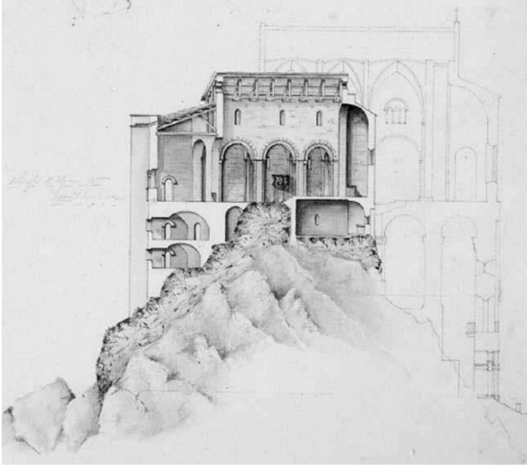
Figure 35 - Hypothetic section of the first church, following d'Andrade Hypothesis Source: Appud Tosco, C. (2023)
