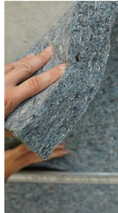
Figure Bt03: Insulation panels made from blue jeans - by Soprema (UK) Source: https://www.soprema.co.uk/en/article/sopravoice/soprema-blue-jeans-sustainable-insulation
