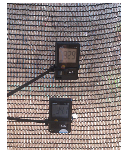
Figure 05.6.15: Testo professional sensors - installed during site survey - one on the outside of the main tent and one on the inside. Source: Picture taken by the author of the thesis
