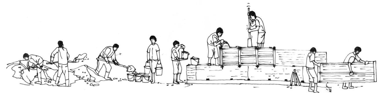
Figure 02.3.4: Building process of rammed earth walls Source: https://madeinearth.in/topics/techniques/rammed-earth/
