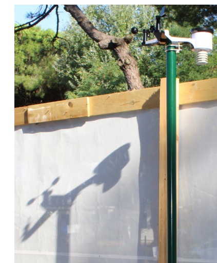
Figure 05.6.16: ICOMAC27 - Micro-climatic station installed on site during the site survey. Source: Picture taken by the author of the thesis
