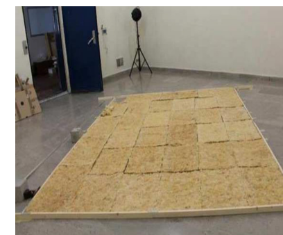
Figure Wo04: Cartonlana - hemp and waste wool insulation panel - by Thiebat et al. (2015)
