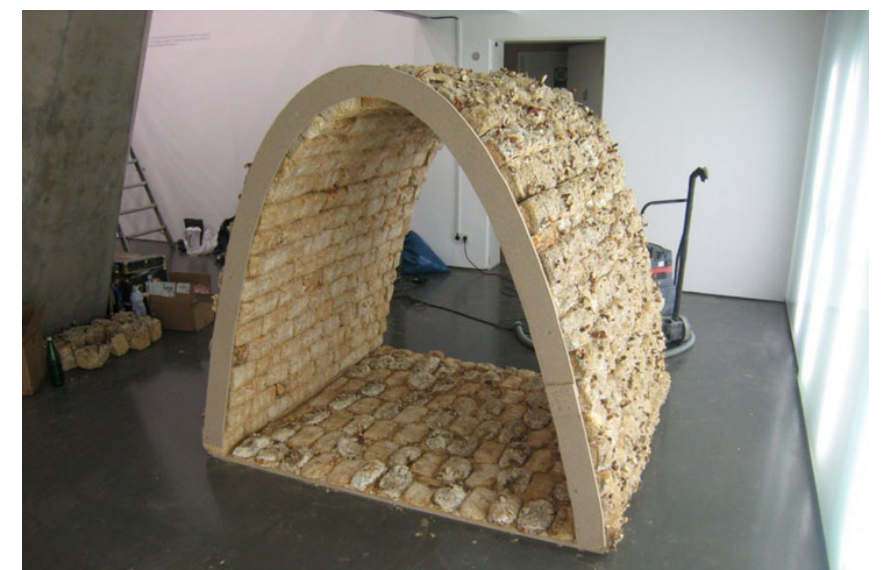
Figure 03.1.3: Ross grew the fungus Ganoderma lucidum (or Reishi) into bricks at the Far West Fungi mushroom farm in Monterey, California Source: https://inhabitat.com
