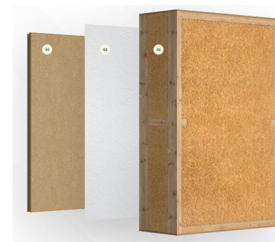
Figure St09: Ecococon prefabricated wall system. 01 6-10 cm fire board, 02 Airtight membrane 03 Timber straw prefabricated panel Source: https://ecococon.eu/the-panel-system
