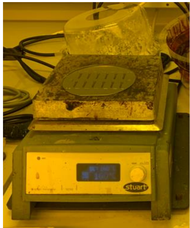
Figure 3.2.12 Hard bake after the development
