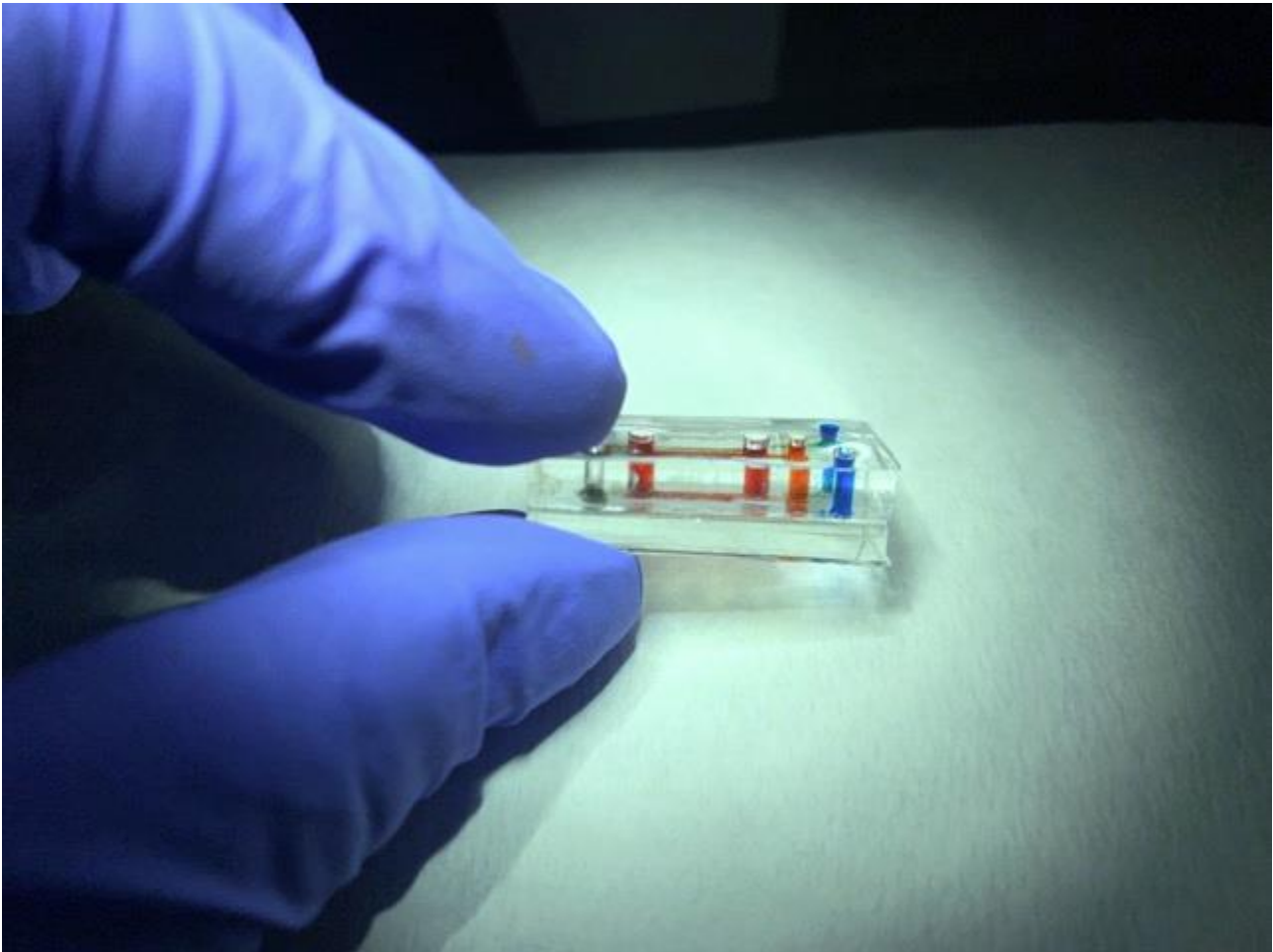
Figure 2.3 Device assembled. External channels in blue and the central channel in orange dye.
