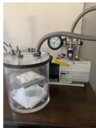
Figure 3.3.2 SYLGARDTM 184 Silicone Elastomer kit (61). Figure 3.3.3 Vacuum pump with PDMS replicas.
