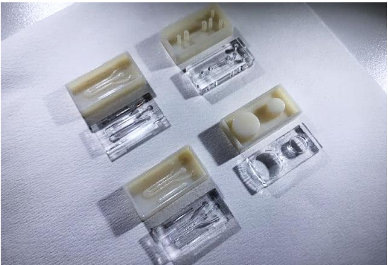
Figure 3.2.2 Molds and replicas of bottom, top and reservoir layers. Molds produced by 3d printing.
