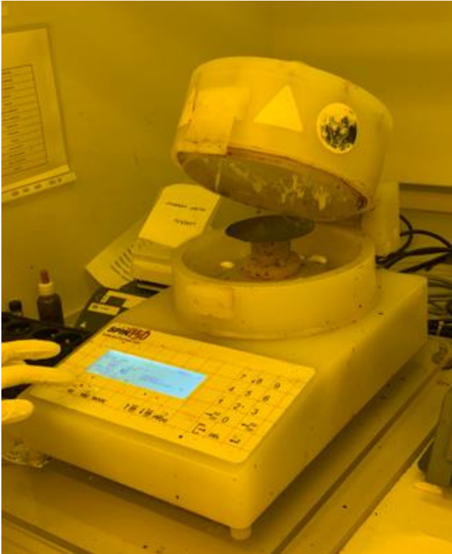
Figure 3.2.9 Spin coater with wafer placed.
