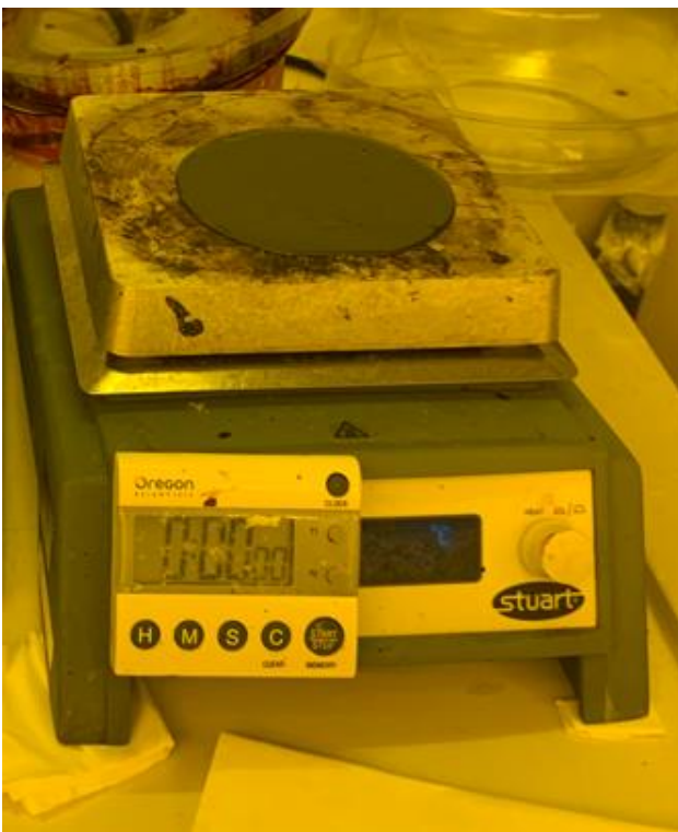
Figure 3.2.11 Post-exposure bake before the development
