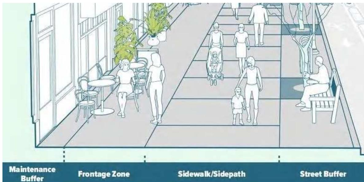
Fig. 2-6 Complete street space elements (Source: Montgomery county complete streets p108)
