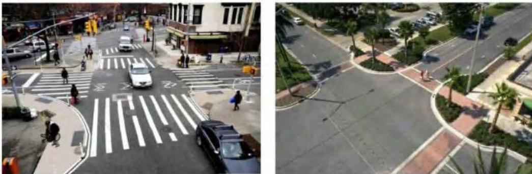
Fig. 4-12 Intersection pavement narrowing and prominent colour intersection pavement(Source:Google)
