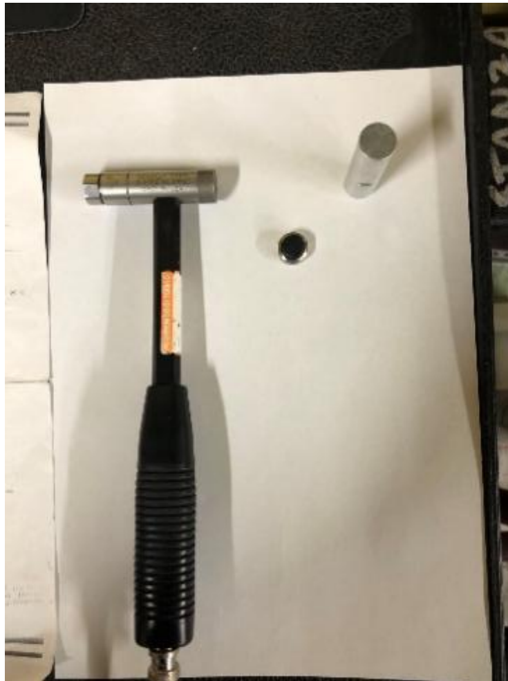
Figure 2.4 Drop hammer and force transduce assembly.
