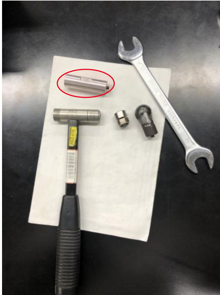
Figure 2.5 The red marking indicates an additional weight block added.
