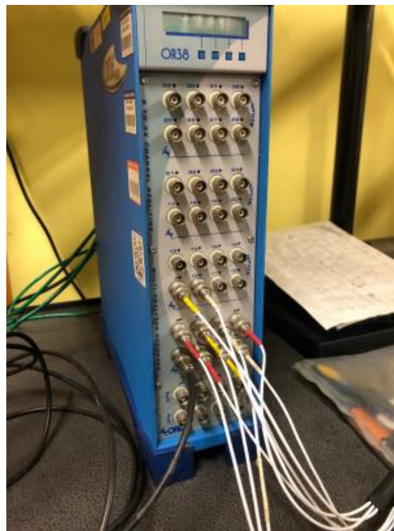
Figure 2.1 the data acquisition system OR38
