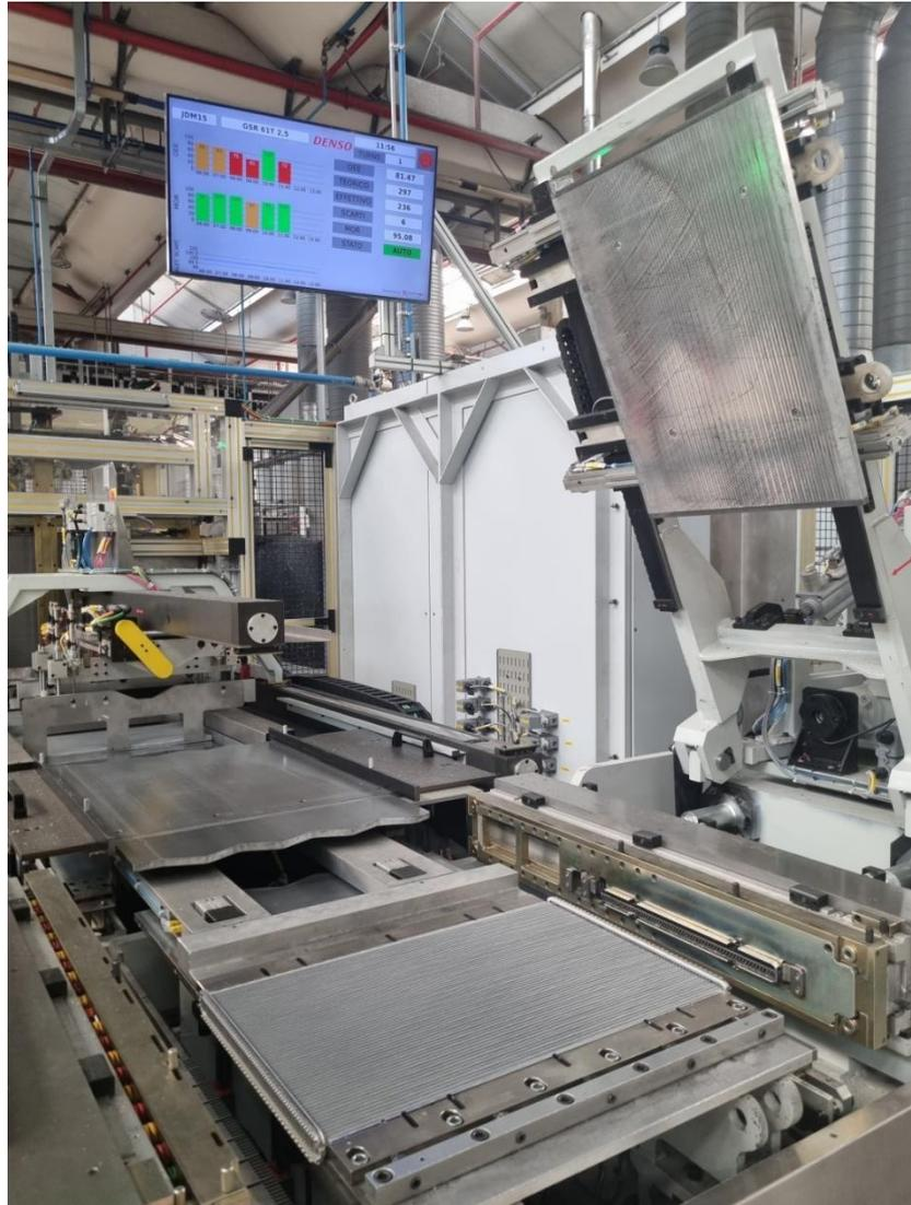
*Figure 13. "JDM" Core builder side*
