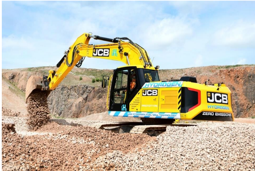
Fig. 0.2 JCB 220X- hydrogen excavator ( JCB's First Hydrogen Powered Excavator | News | JCB.Com, n.d. )
