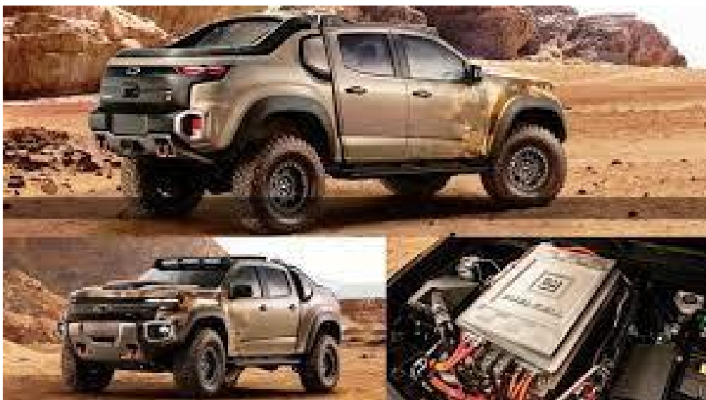
Fig. 0.3 Chevrolet Colorado ZH2- first military vehicle powered by hydrogen fuel cells ( About the Fuel Cell Power Chevy Colorado ZH2| Wright Chevy Buick GMC, 2022/2023 )
