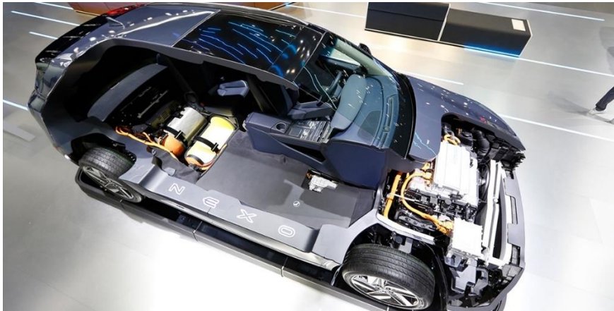
Fig. 1.8 Hyundai Nexo (2019-2022)- Details (Hyundai Goes Full Steam Ahead on Fuel Cell Systems - Electrive.Com, 2022-2023)
