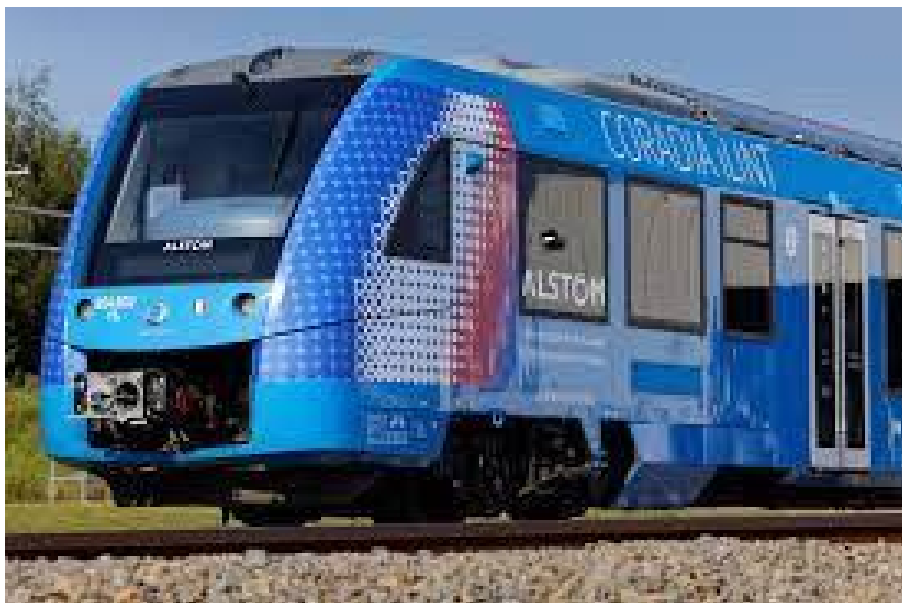
Fig. 1.17 Alstom-Coradia iLint-Hydrail (Alstom's Coradia iLint Hydrogen Train Runs for the First Time in France | Alstom, n.d.)
