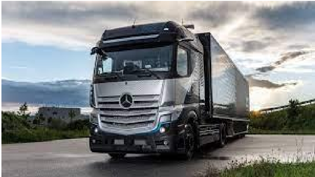
Fig. 1.14 Mercedes-Benz GenH2 Fuel Cell Truck (Daimler and Shell Team up on Hydrogen Trucks, 2022-2023)
