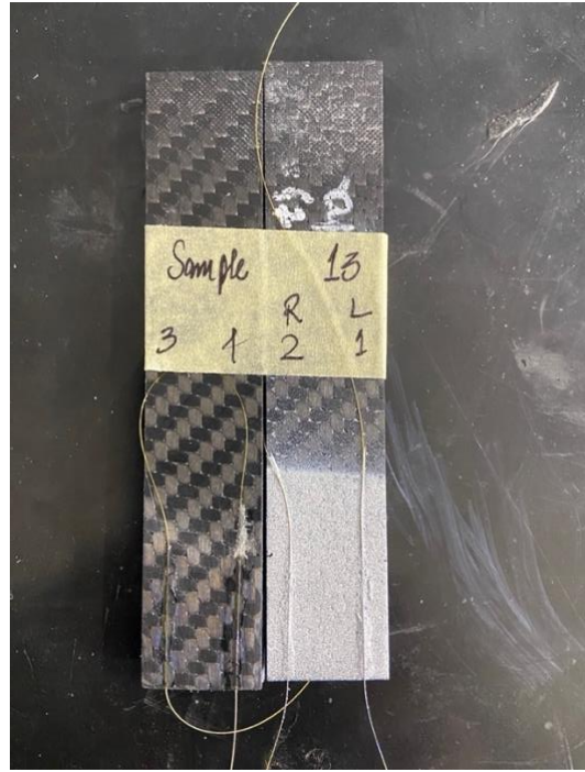
Figure 70. Sample 13 with 20mm overlap
