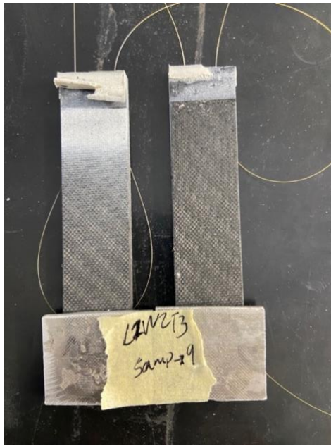
Figure 66. sample 9 with a 10 mm overlap
