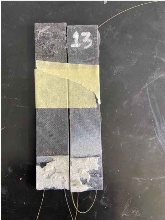
Figure 70. Sample 13 with 20mm overlap
