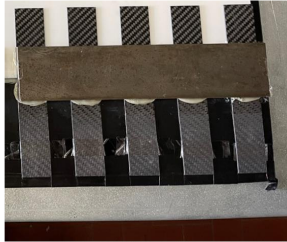
Figure 56. Preparation of SLJ samples for back face strain monitoring
