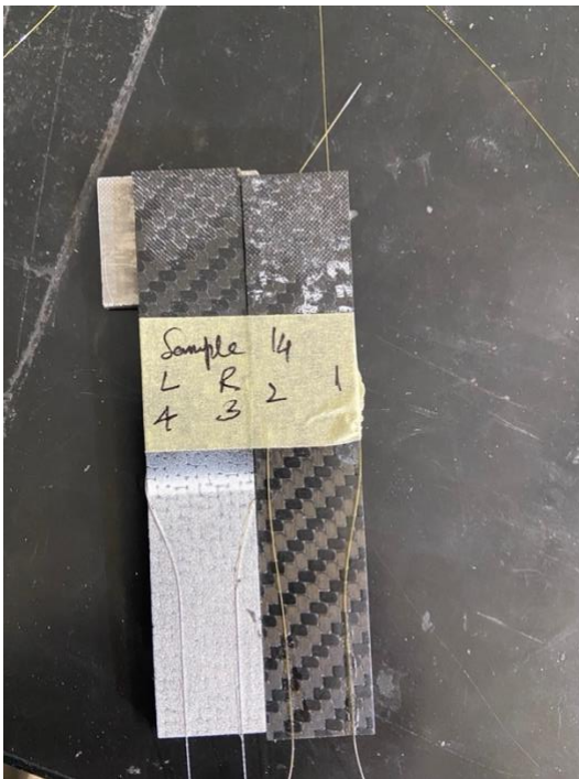
Figure 71. Sample 14 with 20mm overlap
