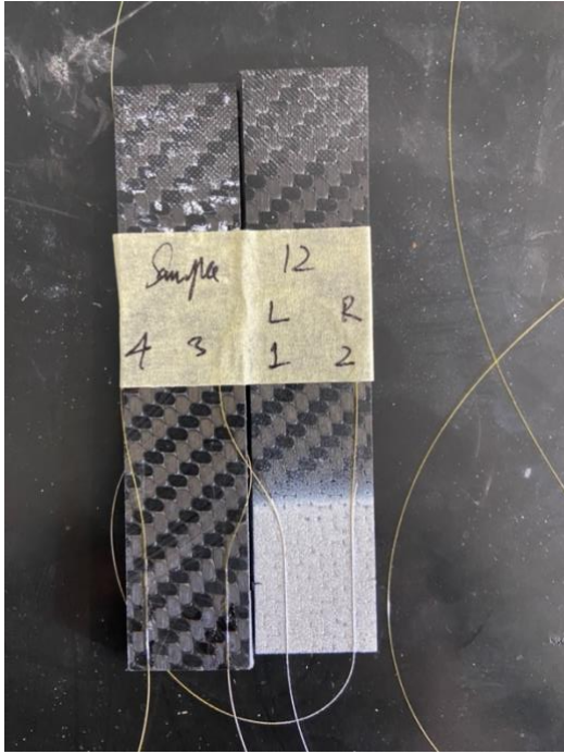
Figure 68. sample 12 with a 10mm overlap
