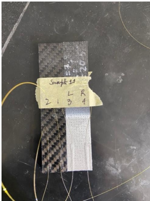
Figure 69. Sample 11 with 20mm overlap
