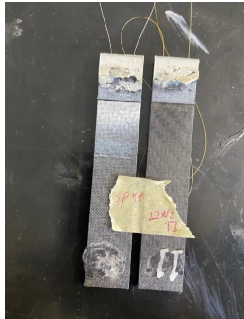
Figure 69. Sample 11 with 20mm overlap
