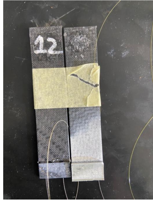
Figure 68. sample 12 with a 10mm overlap
