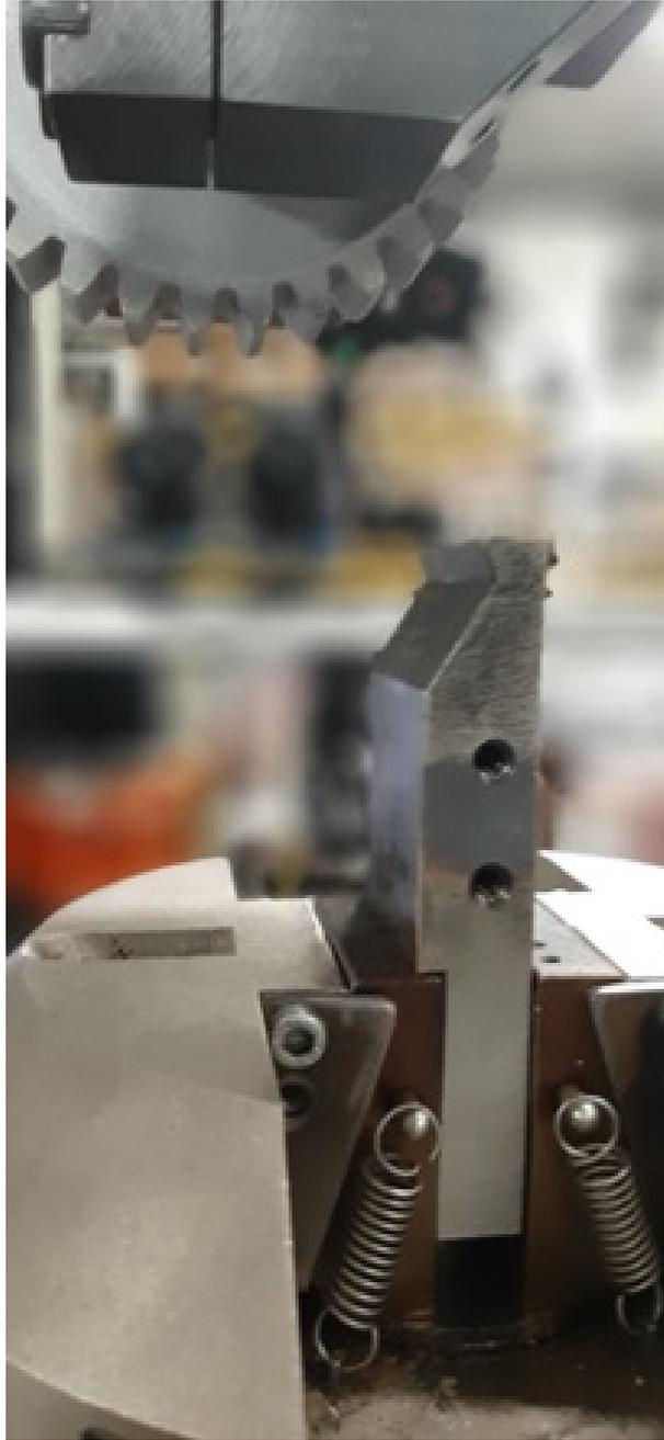
Figure 2.40: The punch that will apply different loads to Standard Gear during the bending test
