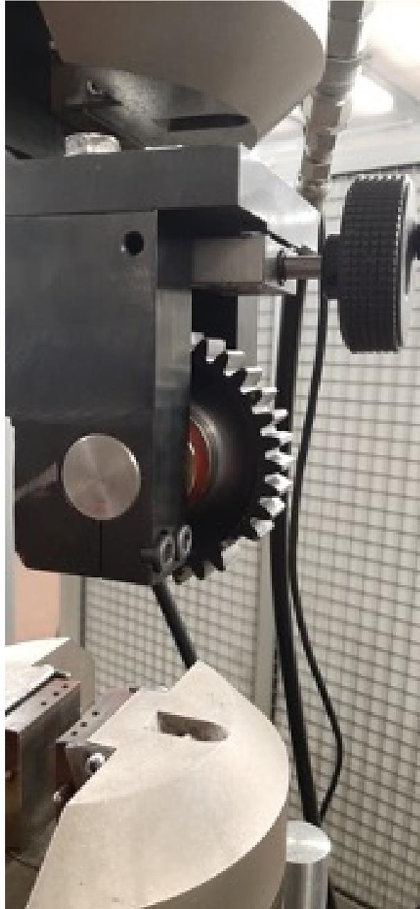
Figure 2.39: Vertical support permanently mounted on the apex of the Instron machine
