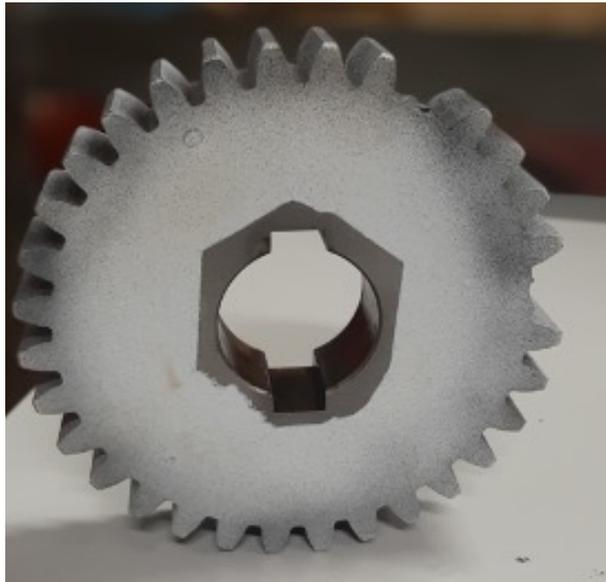
Figure 2.25: Speckled standard gear
