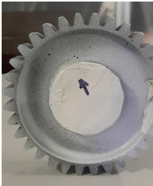
Figure 2.27: Speckled thin-rim gear
