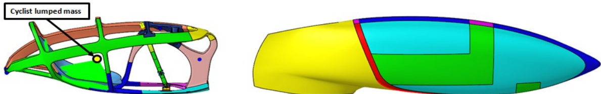
Figure 4.59: (left) Model composed of frame and cyclist lumped mass. (Right) model composed of frame, aerodynamic fairing and cyclist lumped mass.
