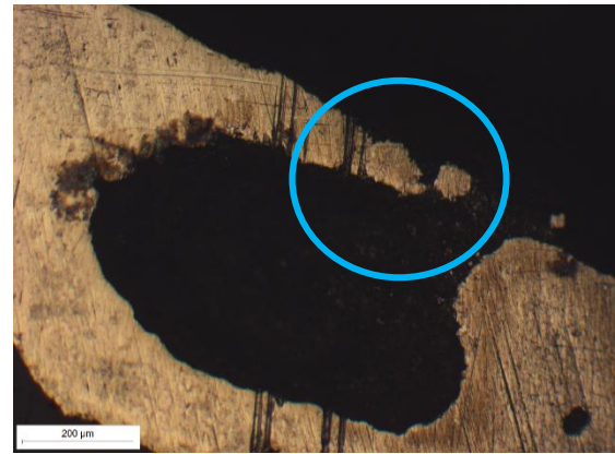
Figure 65 Optical microscopy analysis of aluminum foam of sample 1-B at magnifications of 10x, 20x, and 50x
