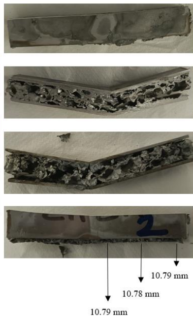
Figure 55 Failure morphology of Sample 2 after 2.7 million loading cycles.
