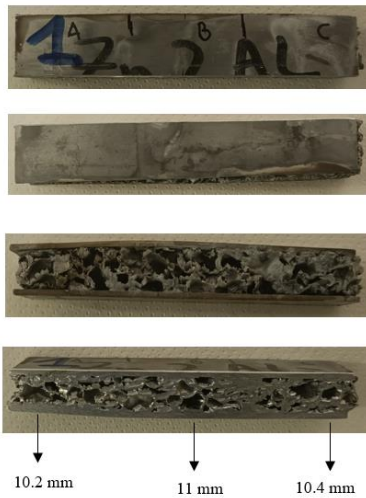
Figure 54 Sample 1 with 4.5 million loading cycles and slight deformation at edges
