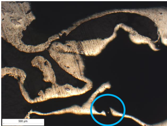
Figure 63 Optical microscopy analysis of aluminum foam of sample 1-A at magnifications of 10x, 20x, and 50x.
