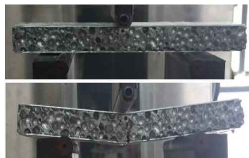
Figure 15 AFS with 304 face sheets under testing [51]
