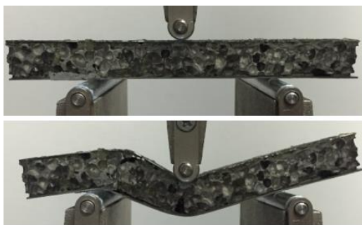
Figure 16 AFS with 6061 face sheets under testing [51]
