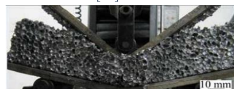
Figure 26 Bending deformation of AFS with 4 mm panel and 50 mm core thickness [53]
