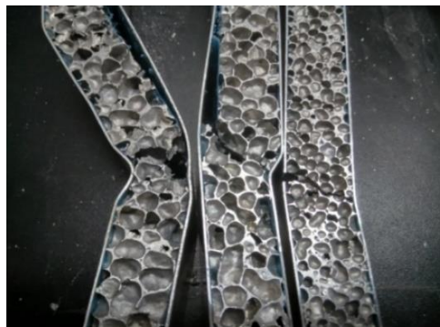
Figure 35 Failure mode of AFS during fatigue tests. a) 0.3 g/cm 3 b) 0.4 g/cm 3 c) 0.6 g/cm 3 [54]
