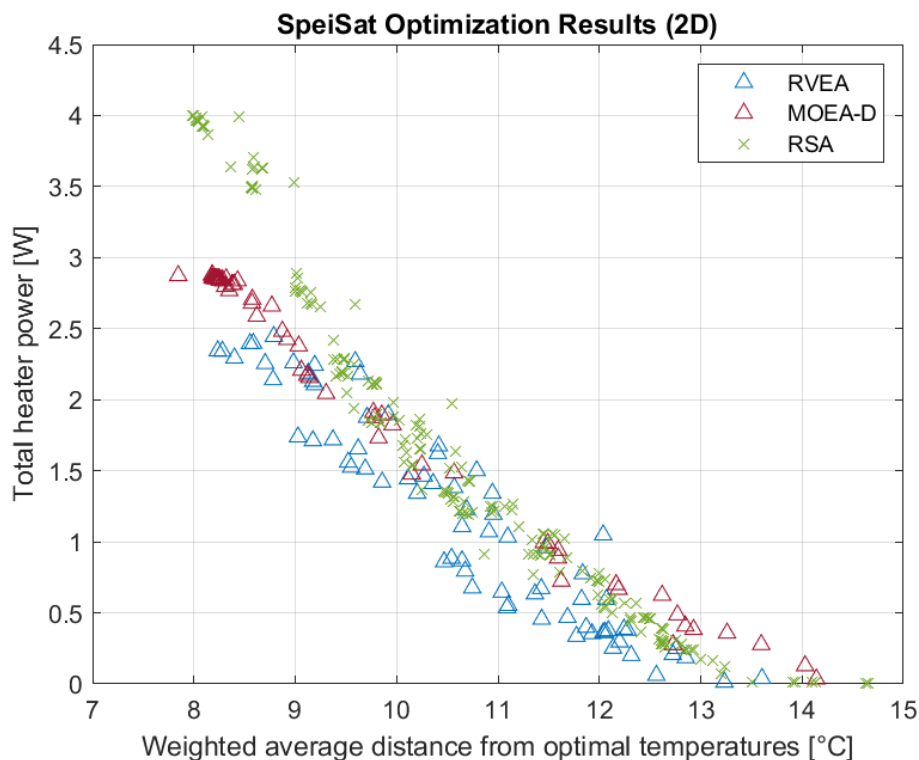
Figure 71: First two objectives (distance from optimal temperatures and total heater power) of the final Pareto fronts generated by RVEA, MOEA/D and RSA in the SpeiSat optimization.
