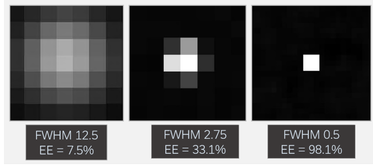
Figure 78: EE in the centroid pixel compared to FWHM
