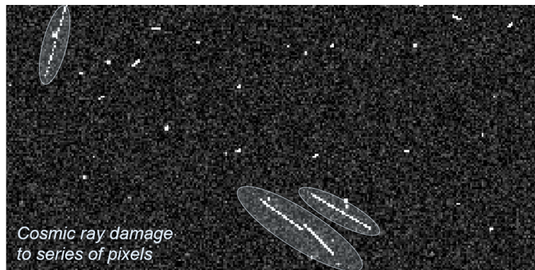
Figure 63: Simulated cosmic ray damage to series and groups of pixel wells
